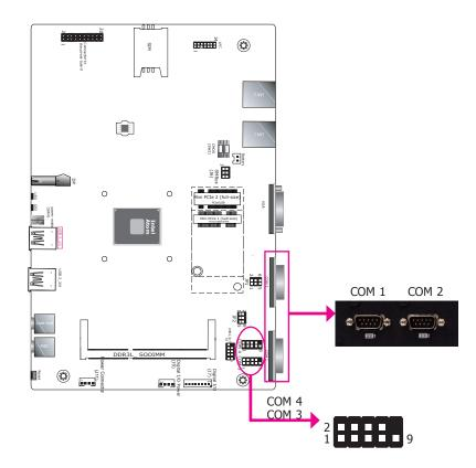
COM 1 to COM 4 can be selected among RS232, 422 and 485. In addition, COM 1 and COM 2 can be selected to supply +12V or +5V power on Pin 9 (default: RI).
