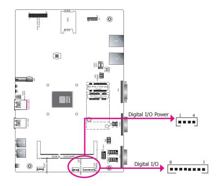
The 8-bit Digital I/O connector provides monitoring and control function to external devices connected to the connector.
