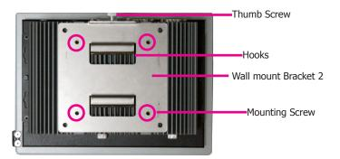
5. Slide the Panel PC to "wall mount bracket 1" to attach the two brackets with the hooks. Then tighten the thumb screw to secure the assembly in place. Note that the following diagram is for illustration only and may not resemble the actual product.
