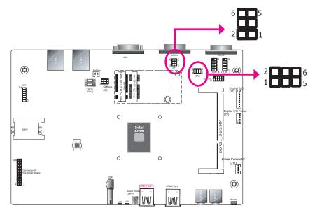
JP1 (for COM 1) and JP2 (for COM 2) are designed to configure the Serial COM ports to provide power. The pin functions of COM 1 and COM 2 will vary according to the jumpers' settings.
