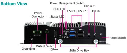
**DC-in Power Connector** Plug a power adapter into this 3-pin terminal block (or optional DC-in jack).
