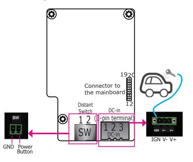
The 3-pole power connector connects to a car battery for power supply. Note that the system accepts a wide power range of 9 to 48V with in-vehicle power management that includes Bat-
