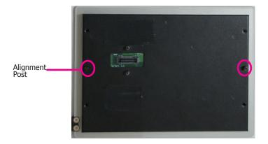
3. Hold the box module with its ADP connector in line with the ADP connector of the panel module. Align the box module with the panel module using the alignment posts.
