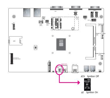
Switch 4 is used to select the power-on mode.
