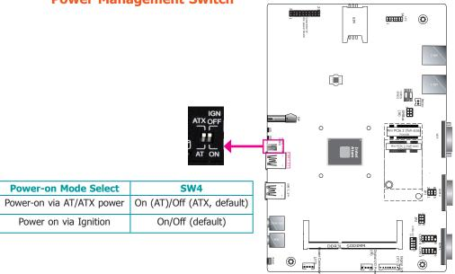
The system powers on via the ignition control with settings of power on/off delay in the BIOS, plus protection from low voltage (i.e. the system will not power on if the car battery's voltage is below 10.5, 21V and 42V for 12V input, 24V and 48V input respectively). Note that for this mode to work, please switch the adjacent AT/ATX mode to ATX first. Also note this mode is not available for systems with a DC-in jack (optional).
