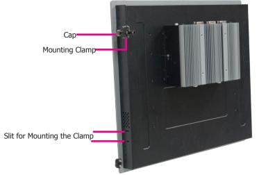
6. The first and second clamps must be positioned and secured diagonally prior to mounting the rest of the clamps. Tighten the clamp's screw using an electric screwdriver by pressing the flat head onto the back of the panel. Note that the following diagram is for illustration only and may not resemble the actual product.
