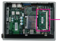
SODIMM Module Installed into the Socket
