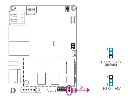
JP1 is used to select the power supplied with the LCD panel.
