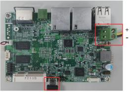
3. Plug in the Micro USB cable to your PC and power-on the FS053.
