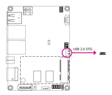
The USB 2.0 OTG port is used for USB communication.
