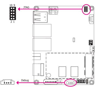
The JTAG and debug connectors are used for debugging purposes.
