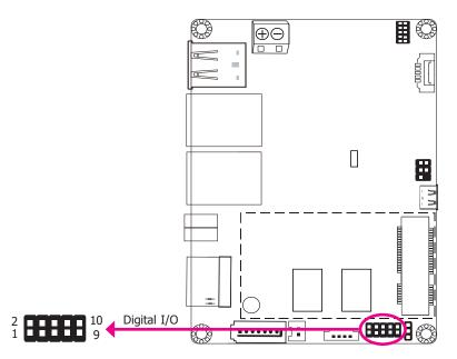
The Digital I/O connector supports 8-bit digital input/output signals to provide powering-on function of the connected devices.
