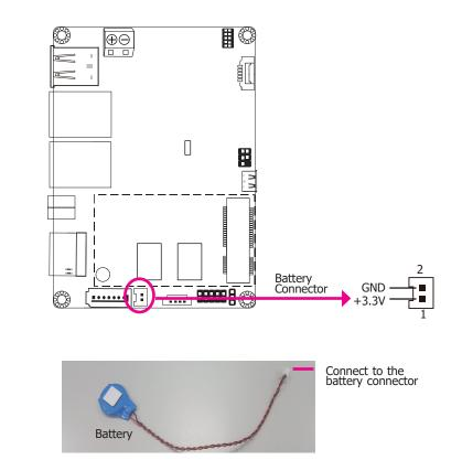
The lithium ion battery powers the real-time clock. It is an auxiliary source of power when the main power is shut off.
