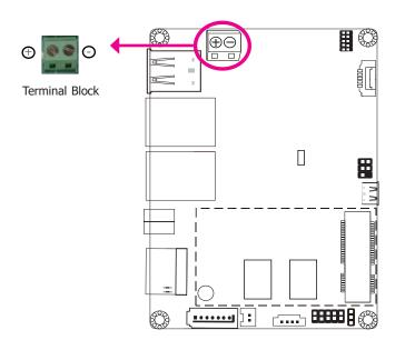
This 2-pin terminal block is considered a low power solution. Connect a DC power cord to this terminal block. Using a voltage more than the recommended range may fail to boot the system or cause damage to the system board.
