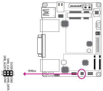
The System Management Bus (SMBus) connector is used to connect SMBus devices. It is a multiple device bus that allows multiple chips to connect to the same bus and enable each one to act as a master by initiating data transfer.
