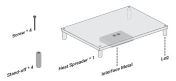
The heat spreader is designed to be mounted onto the module as illustrated below. Please make sure the contacting sides of the heat spreader and the module are correct — the CPU side of the module shall be facing the interface metal side with legs of the heat spreader. Rotate the module horozontally so the interface metal would sit right on top of the CPU.
