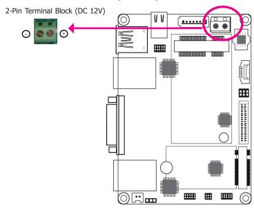
This 2-pin terminal block is considered a low power solution. Connect a power adapter and a 2-pole terminal to DC Jack cable to this terminal block. Using a voltage more than the recommended range may fail to boot the system or cause damage to the system board.
