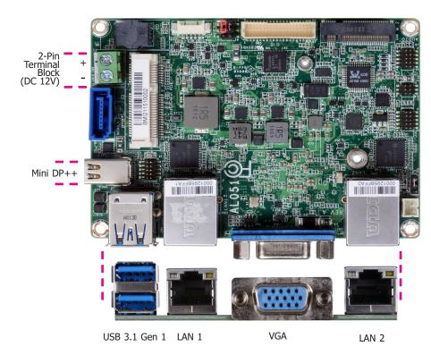
The rear panel I/O consists of the following ports:
