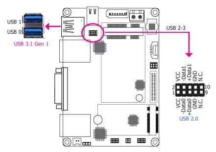
The USB device allows data exchange between your computer and a wide range of simultaneously accessible external Pluq and Play peripherals.
