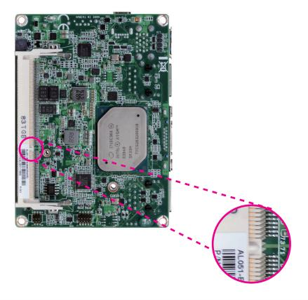
Grasping the module by its edges, align the module into the socket at an approximately 30 degrees angle. Apply firm even pressure to each end of the module until it slips down into the socket. The contact fingers on the edge of the module will almost completely disappear inside the socket.
