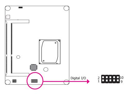
The Digital I/O connector supports 8-bit digital input/output signals to provide the ability of monitoring and controlling the states of the connected external devices.
