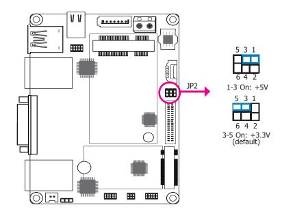
JP2 is used to select the power supplied with the LCD panel.
