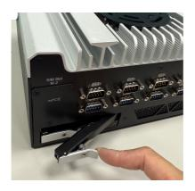
Step 3: Slide the drive into the slot until the drive is fully seated. Close the drive latch to lock the drive in place.
