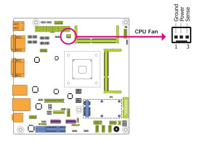
The fan connector is used to connect the cooling fan. The cooling fan will provide adequate airflow throughout the chassis to prevent overheating the CPU and system board components.
