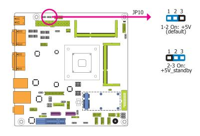
JP10 is used to select the power of the PS/2 keyboard/mouse port. Selecting +5V\_standby will allow you to use the PS/2 keyboard or PS/2 mouse to wake up the system.
