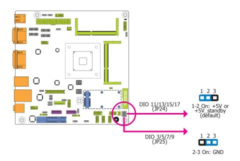
Based on the power level of DIO (Digital I/O) selected on JP23, JP25 (DIO pin 3/5/7/9) and JP24 (DIO pin 11/13/15/17) are used to select the output state of Digital I/O: pull high or pull low. When selecting pull high, the power selection will be the same as JP23's setting.
