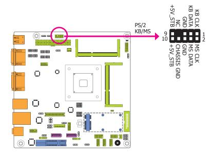
The Keyboard/Mouse connector is used to connect PS/2 keyboard and PS/2 mouse by means of a PS/2 cable. Connect one end of the cable to the Keyboard/Mouse connector. The other ends are used to connect a PS/2 keyboard and a PS/2 mouse.
