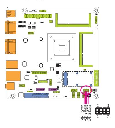
These LAN LED connector is used to detect the connection state of RJ45 LAN ports when the connection is made to an active network via a cable. The pin functions of the LAN LED connector are listed below.
