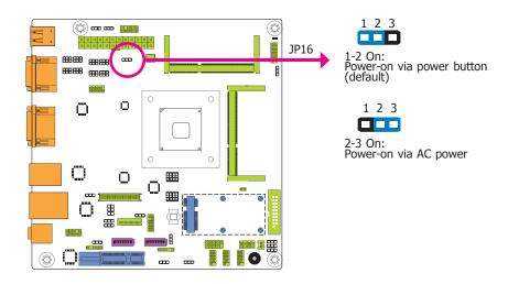
JP16 is used to select the method of powering on the system. If you want the system to power-on whenever AC power comes in, set JP16 pins 2 and 3 to On. If you want to use the power button, set pins 1 and 2 to On.
