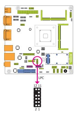
The LPC connector is used for the debug function and its pin functions are listed below.
