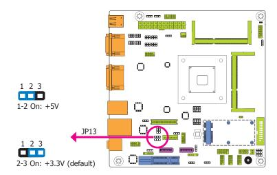
JP13 is used to select the power level of backlight brightness control: +5V or +3.3V.
