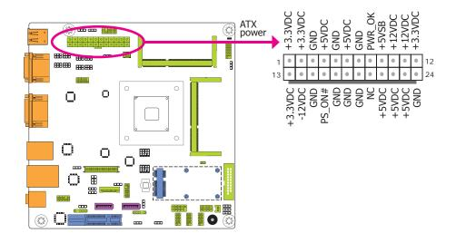
Use a power supply that complies with the ATX +12V Power Supply Design Guide Version 1.1. An ATX +12V power supply unit has a standard 24-pin ATX main power connector that must be inserted into the 24-pin connector.
