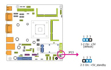
JP23 is used to select the power of Digital I/O signal.
