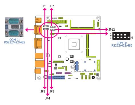
These jumpers allow you to configure the Serial COM ports to RS232, RS422 (Full Duplex) or RS485. JP1, JP2 and JP4 are used to configure the Serial COM port 1. JP7, JP8 and JP12 are used to configure the Serial COM port 3. The pin functions of Serial COM port 1 and COM port 3 will vary according to these jumpers' setting.
