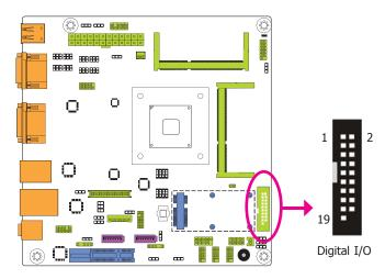
The 8-bit Digital I/O connector provides powering-on function to external devices that are connected to these connectors. The pin functions of the 8-bit digital I/O connector are listed below.
