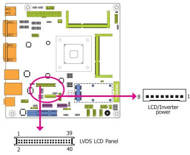
The system board allows you to connect a LCD Display Panel by means of the LVDS LCD panel connector and the LCD/Inverter power connector. These connectors transmit video signals and power from the system board to the LCD Display Panel.
