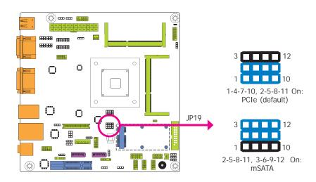
JP19 is used to select the Mini PCIe signal: PCIe or mSATA.
