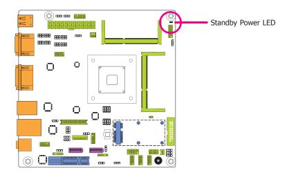
This LED will light red when the system is in the standby mode. It indicates that there is power on the system board. Power-off the PC and then unplug the power cord prior to installing any devices. Failure to do so will cause severe damage to the motherboard and components.
