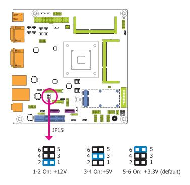
JP15 is used to select the power supplied with the LCD panel.
