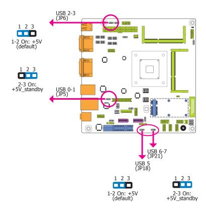
JP5, JP6, JP18 and JP21 are used to select the power of the USB ports. Selecting +5V\_standby will allow you to use a USB device to wake up the system.
