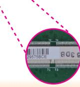
Grasping the module by its edges, align the module into the socket at an approximately 30 degrees angle. Apply firm even pressure to each end of the module until it slips down into the socket. The contact fingers on the edge of the module will almost completely disappear inside the socket.
