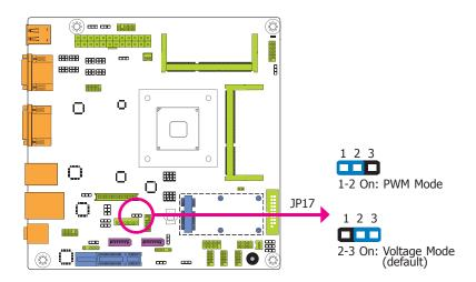
JP17 allows you to select the mode for the lightness control of the LVDS panel.
