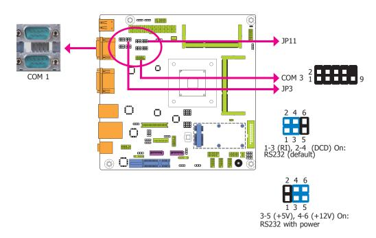
JP3 (for COM 1) and JP11 (for COM 3) are used to configure the Serial COM ports to pure RS232 or RS232 with power.
