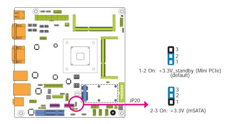
JP20 is used to select the power supplied with the Mini PCIe.
