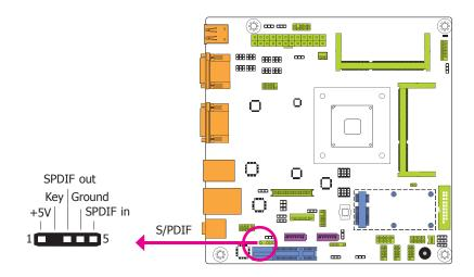
The S/PDIF connector is used to connect an external S/PDIF port. Your S/PDIF port may be mounted on a card-edge bracket. Install the card-edge bracket to an available slot at the rear of the system chassis then connect the audio cable to the S/PDIF connector. Make sure pin 1 of the audio cable is aligned with pin 1 of the S/PDIF connector.
