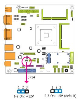
JP14 is used to select the power level of the LCD/inverter power connector.
