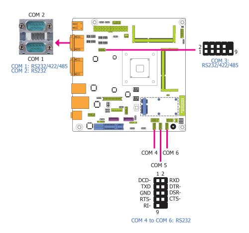
COM 2, COM 4, COM 5 and COM 6 are fixed at RS232.
