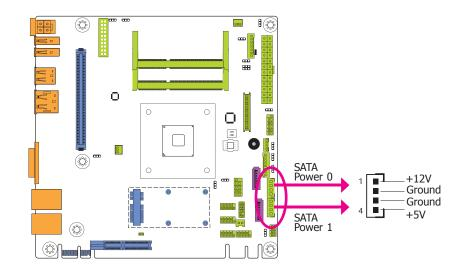
These SATA power connectors supply power to the SATA drive. Connect one end of the provided power cable to the SATA power connector and the other end to your storage device.
