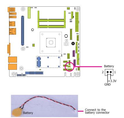
The lithium ion battery powers the real-time clock and CMOS memory. It is an auxiliary source of power when the main power is shut off.
