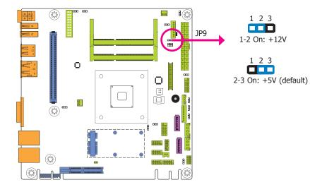
JP9 is used to select the power level of the LCD/Inverter power connector.
