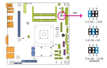
JP8 is used to select the power supplied with the LCD panel.
