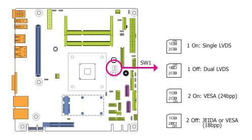
The Switch 1 is used to select the LVDS channel and the color of bits per pixel on the system.
