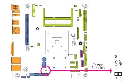
The board supports the chassis intrusion detection function. Connect the chassis intrusion sensor cable from the chassis to this connector. When the system's power is on and a chassis intrusion occurred, an alarm will sound. When the system's power is off and a chassis intrusion occurred, the alarm will sound only when the system restarts.
