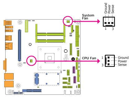
The fan connectors are used to connect cooling fans. The cooling fans will provide adequate airflow throughout the chassis to prevent overheating the CPU and system board components.
