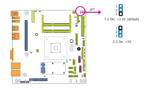
JP7 is used to select the power level of backlight control: +3.3V (default) or +5V.
