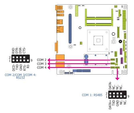
COM 1 is fixed at RS485 and COM 2 to COM 4 are fixed at RS232.
