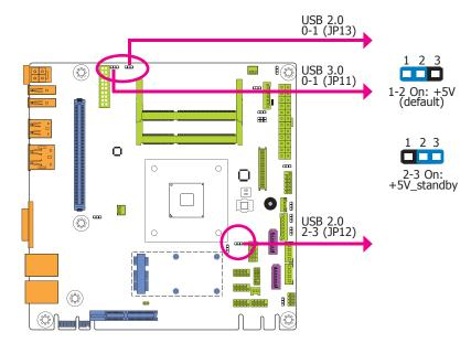
JP11, JP12 and JP13 are used to select the power of the USB ports. Selecting +5V\_standby will allow you to use a USB device to wake up the system.
