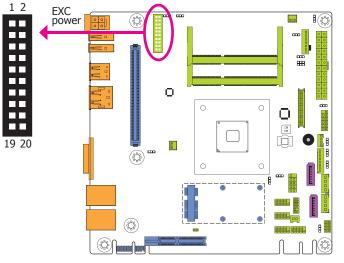
The EXC power connector provides the power supplement for an EXC card to operate when the EXC card is installed into the EXC interface. The pin functions of the EXC power connector are listed below.
