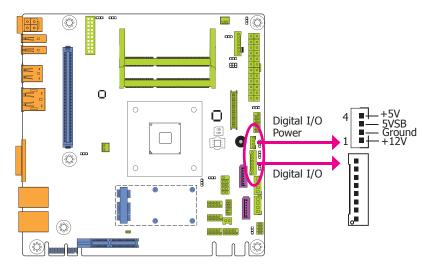
The 8-bit Digital I/O connector provides powering-on function to external devices that are connected to these connectors.
