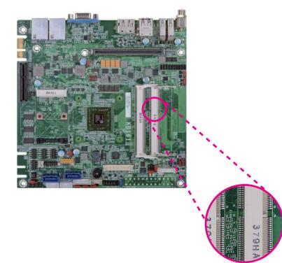
5. Grasping the module by its edges, align the module into the socket at an approximately 30 degrees angle. Apply firm even pressure to each end of the module until it slips down into the socket. The contact fingers on the edge of the module will almost completely disappear inside the socket.
