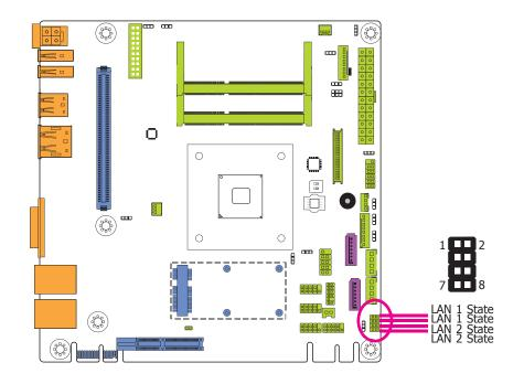
The LAN LED connector is used to detect the connection state of RJ45 LAN ports when the connection is made to an active network via a cable. The pin functions of the LAN LED connector are listed below.
