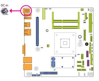
This jack provides maximum of 100W power and is considered a low power solution. Connect a DC power cord to this jack. Use a power adapter with 12V DC output voltage. Using a voltage higher than the recommended one may fail to boot the system or cause damage to the system board.
