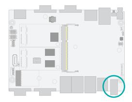
The 9~36V DC-In coaxial supports wide-range voltage power connection.
