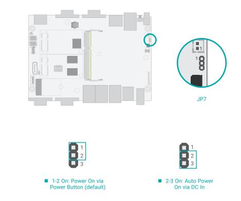
The jumper allows you to choose between system power-on via power button and automatic power-on via DC power in.
