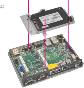
4. Connect the SATA cable and the SATA power cable to the SSD and the board connectors.
