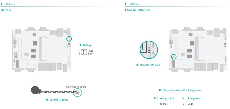
The external lithium ion battery supplies power to the real-time clock and CMOS memory as an auxiliary source of power when the main power is shut off.
