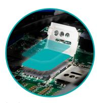
Step 3: Orient the SIM card and place it into the socket.
