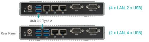
USB allows data exchange between your computer and a wide range of simultaneously accessible external Plug and Play peripherals. The system board is equipped with multiple USB Type A ports at the front panel – two USB 3.0 or four USB 3.0 ports – along with two internal USB 2.0 pin-header ports.
