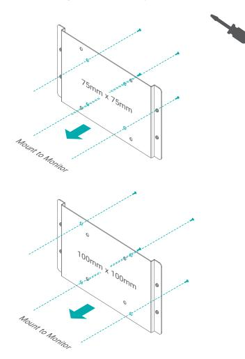
Attache the brackets to the bottom side of the system as illustrated below.
