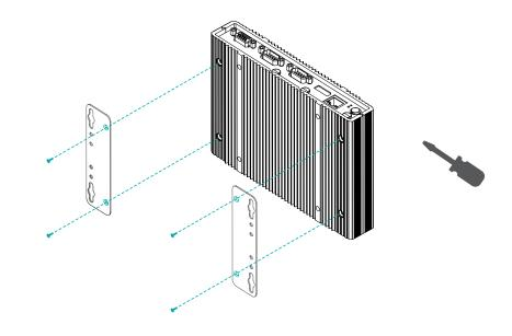
Mount the assembly onto the VESA mount bracket previously attached to the back of a monitor.
