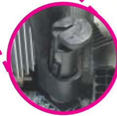
"Unlocked" position of push-pin
