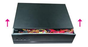
5. The DIMM sockets and SATA drive bay are readily accessible after removing the chassis cover.
