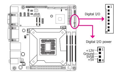
The 8-bit Digital I/O connector provides the ability of monitoring and control of the connected external devices.
