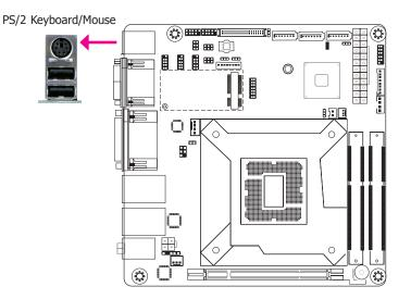
This rear I/O port is used to connect a PS/2 keyboard/mouse.
