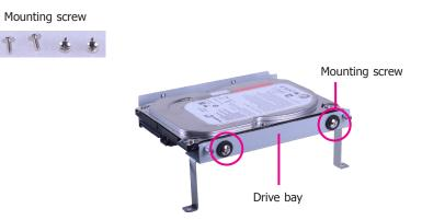
4. Place the drive bay back in the chassis and install the drive bay using the mounting screws you removed in step 1.
