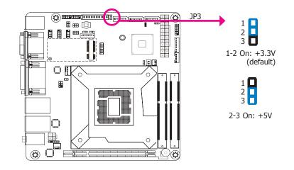
JP3 is used to select the power level of backlight brightness control: +3.3V or +5V.
