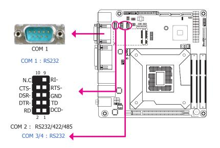
COM 1, COM 3 and COM 4 are fixed at RS232 whereas COM 2 can be selected among RS232/422/485 using the BIOS setup utility.
