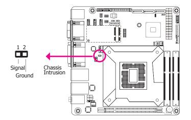
The board supports the chassis intrusion detection function. Connect the chassis intrusion sensor cable from the chassis to this connector. When the system's power is on and a chassis intrusion occurred, an alarm will sound. When the system's power is off and a chassis intrusion event occurs, the alarm will sound only after the system restarts.
