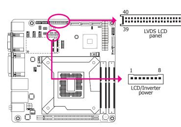
The system board allows you to connect a LCD Display Panel by means of the LVDS LCD panel connector and the LCD/Inverter power connector. These connectors transmit video signals and power from the system board to the LCD Display Panel.
