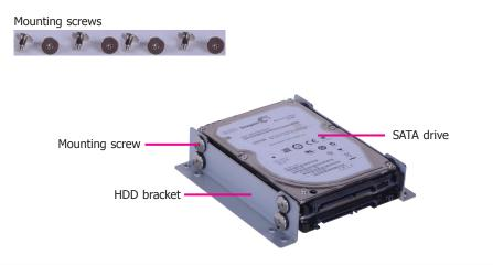
3. Use the provided mounting screws to attach the HDD bracket to the drive bay.
