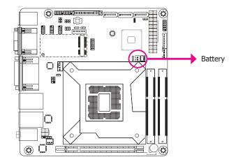
The lithium ion battery powers the real-time clock and CMOS memory. It is an auxiliary source of power when the main power is shut off.
