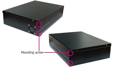
2. Use the provided mounting screws to secure the wall mount brackets on each side of the system.
