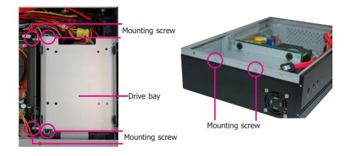
2. Align the mounting holes on the SATA drive with the mounting holes on the HDD bracket and use the mounting screws provided in the drive bay kit to secure the drive in place.
