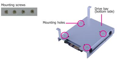
4. Place the SATA drive bay back in the chassis and install the SATA drive bay using the mounting screws you removed in step 1.
