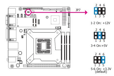
JP7 is used to select the power supplied with the LCD panel.
