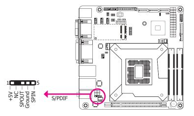
S/PDIF (Sony/Philips Digital Interface Format), a type of digital audio connector, is used for digital audio transmission or output.
