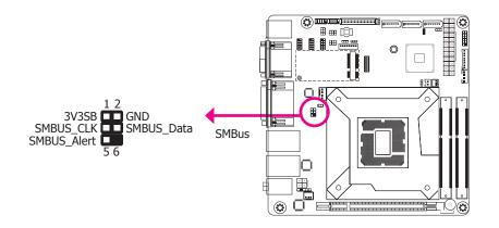
The SMBus (System Management Bus) connector is used to connect SMBus devices. It is a multiple device bus that allows multiple chips to connect to the same bus and enable each one to act as a master by initiating data transfer.
