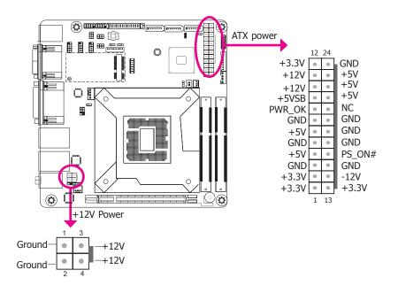
Use a power supply that complies with the ATX12V Power Supply Design Guide Version 1.1. An ATX12V power supply unit has a standard 24-pin ATX main power connector that must be inserted into the 24-pin connector. The 4-pin +12V power connector enables the delivery of more +12VDC current to the processor's Voltage Regulator Module (VRM).
