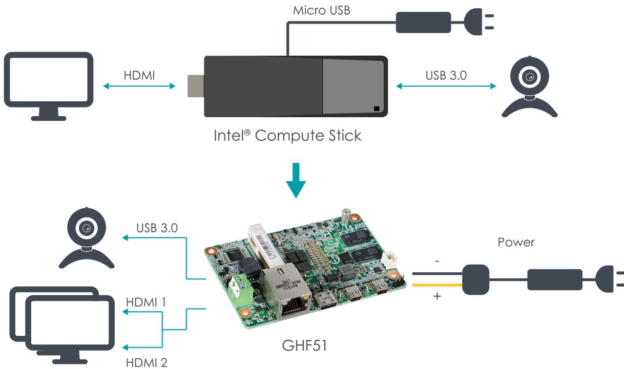
and Digital I/O that is not provided by ordinary personal computers. Its powerful flexibility and versatility can better meet future requirements, such as dual-screen systems, high-speed networking, and control systems connected with many peripheral devices through DIO Link, extending to access control or smart home system.
