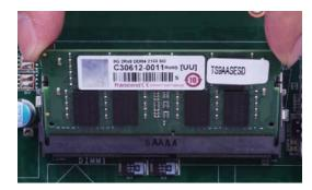
6. Push down the module until the clips at each end of the socket lock into position. You will hear a distinctive "click", indicating the module is correctly locked into position.
