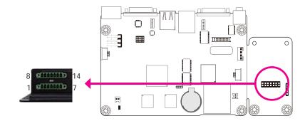
The Digital I/O connector provides powering-on function to an external device that is connected to this connector.
