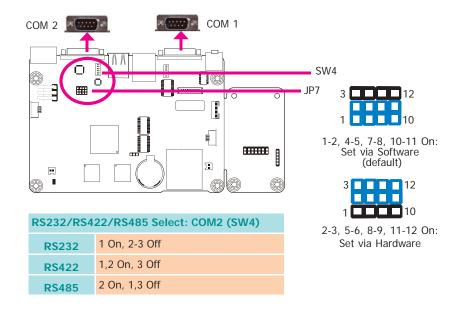
SW4 (for COM2) is used to configure the COM port to RS232, RS422 (Full Duplex) or RS485.
