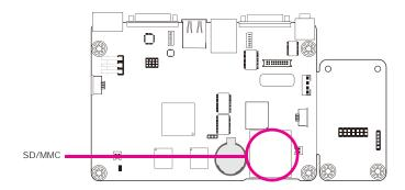
This expansion port is used to insert a Secure Digital (SD) or Multimedia Card (MMC) device. Aside from storing data files, an SD card is also capable of storing powerful software applications
