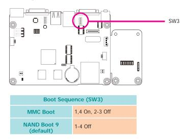
SW3 is used to configure the boot sequence of system.
