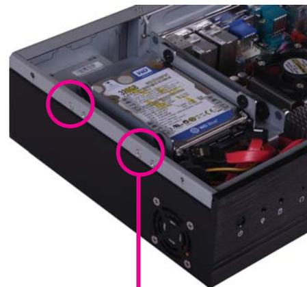
6. Connect the SATA data cable and SATA power cable to the connectors on the SATA drive.
