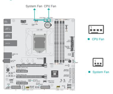
These fan connectors are used to connect cooling fans. The cooling fans will provide adequate airflow throughout the chassis to prevent overheating the CPU and system board components.
