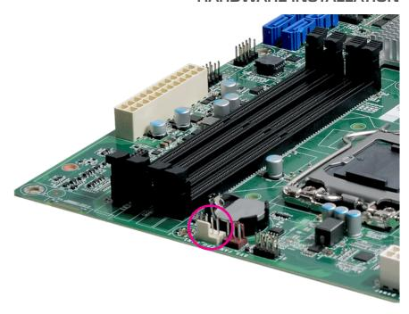
Align the 4 screw holes and tighten the heat sink up by inserting screws, D0 remember to connect the fan cable on the board. (The location of fan connector may vary.)
