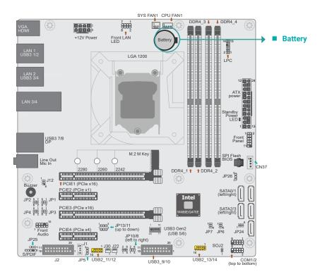
The lithium ion battery addendum supplies power to the real-time clock and CMOS memory as an auxiliary source of power when the main power is shut off. Insert a coin cell battery into the holder and make sure the polarities are correctly oriented – the cap side (rimmed rounded edge) is negative and should be facing the holder; the flat side with a + mark is positive and should be facing away from the holder.
