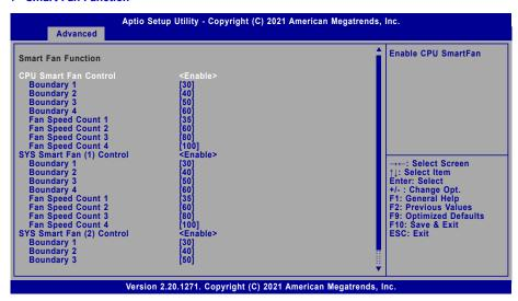
Smart Fan is a fan speed moderation strategy dependent on the current system temperature. When the system temperature goes higher than the Boundary setting, the fan speed will be turned up to the setting of the Fan Speed Count that bears the same index as the Boundary field.
