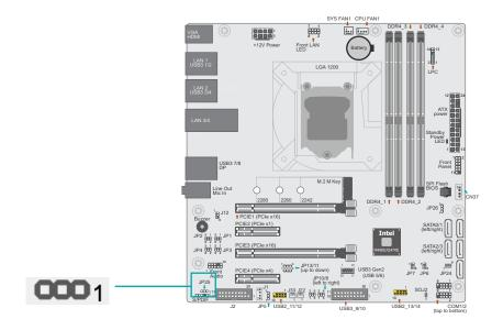
JP25 is used to determine the USB power.
