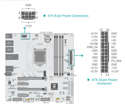
Use a power supply that complies with the ATX12V Power Supply Design Guide Version 1.1. An ATX12V power supply unit has a standard 24-pin ATX main power connector that must be inserted into the 24-pin connector. The 8-pin +12V power connector enables the delivery of more +12VDC current to the processor's Voltage Regulator Module (VRM).
