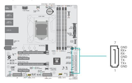
The Serial ATA (SATA) connectors are used to connect the Serial ATA device. SATA 3.0 is supported by the five SATA ports and provides data rate up to 6Gb/s. Connect one end of the Serial ATA cable to a SATA connector and the other end to your Serial ATA device.
