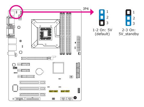
JP4 is used to select the power of the PS/2 keyboard/mouse port. Selecting  $5V_{standby}$  will allow you to use the PS/2 keyboard or PS/2 mouse to wake up the system.
