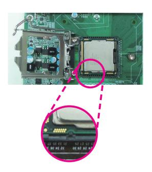
8. Close the load plate then push the load lever down.
