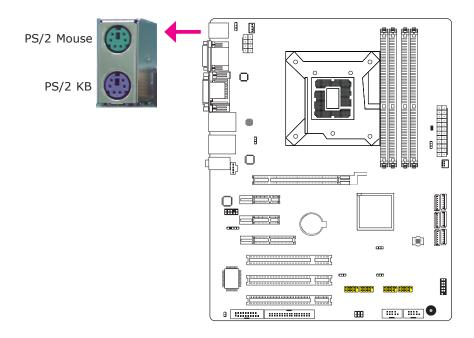
These ports are used to connect a PS/2 mouse and a PS/2 keyboard. The PS/2 mouse port uses IRQ12.
