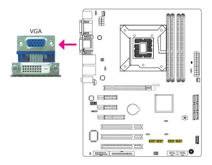
The VGA port is used for connecting a VGA monitor. Connect the monitor's 15-pin D-shell cable connector to the VGA port. After you plug the monitor's cable connector into the VGA port, gently tighten the cable screws to hold the connector in place.
