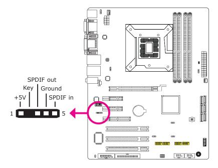
The S/PDIF connector is used to connect an external S/PDIF port. Your S/PDIF port may be mounted on a card-edge bracket. Install the card-edge bracket to an available slot at the rear of the system chassis then connect the audio cable to the S/PDIF connector. Make sure pin 1 of the audio cable is aligned with pin 1 of the S/PDIF connector.
