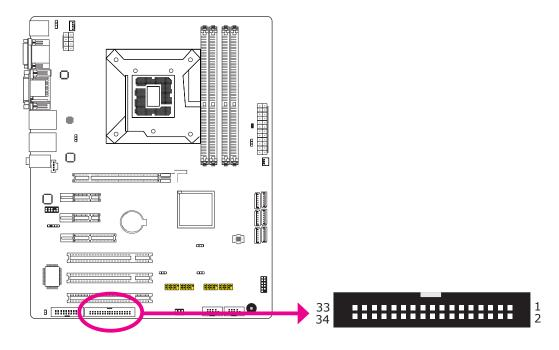
The FDD connector supports a standard floppy disk drive. The floppy cable can be inserted into this connector only if pin 1 of the cable is aligned with pin 1 of this connector.
