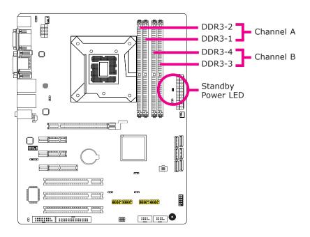
The four DIMM sockets are divided into 2 channels:
