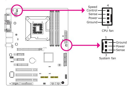
The fan connectors are used to connect cooling fans. The cooling fans will provide adequate airflow throughout the chassis to prevent overheating the CPU and system board components.
