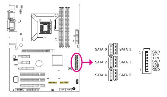
The Serial ATA connectors are used to connect Serial ATA devices. Connect one end of the Serial ATA cable to a SATA connector and the other end to your Serial ATA device.
