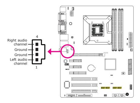
The CD-in connector is used to receive audio from a CD-ROM drive, TV tuner or MPEG card.
