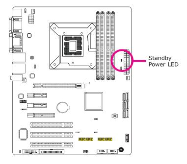
This LED will lit red when the system is in the standby mode. It indicates that there is power on the system board. Power-off the PC then unplug the power cord prior to installing any devices. Failure to do so will cause severe damage to the motherboard and components.
