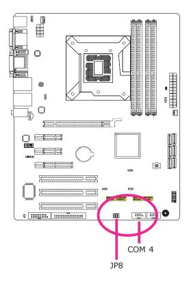
JP8 is used to configure COM 4 to RS232 or RS485.
