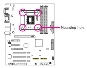
Orient the heat sink such that the CPU fan's cable is nearest the CPU fan connector.
