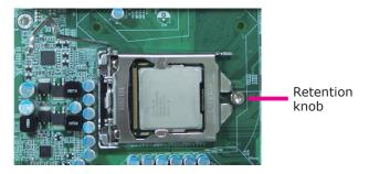
9. Hook the load lever under the retention tab.
