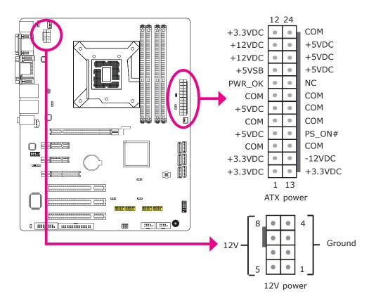
Use a power supply that complies with the ATX12V Power Supply Design Guide Version 1.1. An ATX12V power supply unit has a standard 24-pin ATX main power connector that must be inserted into the 24-pin connector. The 8-pin +12V power connector enables the delivery of more +12VDC current to the processor's Voltage Regulator Module (VRM).
