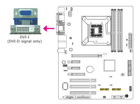
The DVI-I port is used to connect an LCD monitor. This port supports DVI-D signal only.
