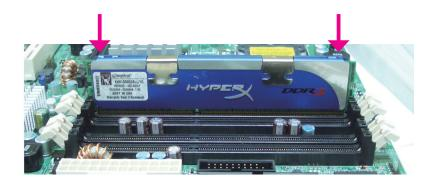
8. The ejector tabs at the ends of the socket will automatically snap into the locked position to hold the module in place.
