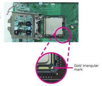
The CPU's notch will at the same time fit into the socket's alignment key.
