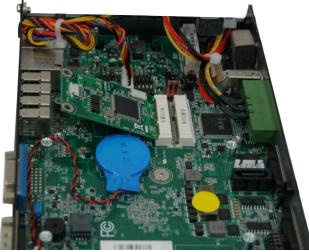
2. Push the Mini PCIe card down and use the provided mounting screws to secure the card on the system board.
