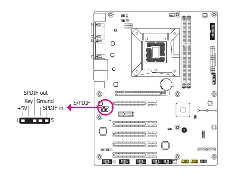
The S/PDIF connector is used to connect an external S/PDIF port. Your S/PDIF port may be mounted on a card-edge bracket. Install the card-edge bracket to an available slot at the rear of the system chassis then connect the audio cable to the S/PDIF connector. Make sure pin 1 of the audio cable is aligned with pin 1 of the S/PDIF connector.
