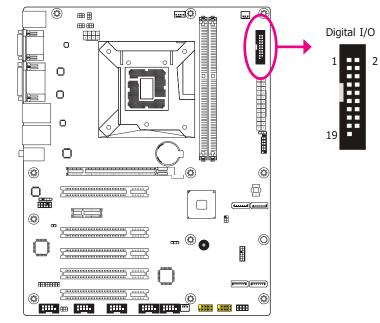
The 8-bit Digital I/O connector provides powering-on function to external devices that are connected to these connectors.
