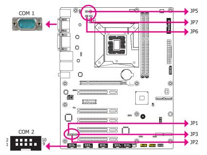
JP5/JP6/JP7 (for COM1) and JP1/JP2/JP3 (for COM2) are used to configure the COM ports to RS232, RS422 (Full Duplex) or RS485. When COM 1 RS232/422/485 is selected, JP6 and JP7 must be set in accordance to JP5. When COM 2 RS232/422/485 is selected, JP2 and JP3 must be set in accordance to JP1. The pin functions of the COM ports will vary according to the jumpers' setting.
