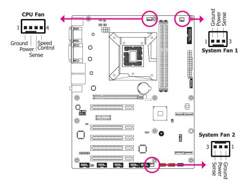
These fan connectors are used to connect cooling fans. The cooling fans will provide adequate airflow throughout the chassis to prevent overheating the CPU and system board components.
