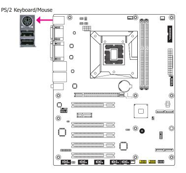
This rear I/O port is used to connect a PS/2 keyboard/mouse. The PS/2 mouse port uses IRQ12.
