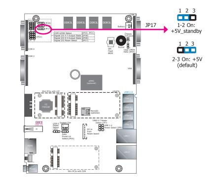
JP17 is used to select the power of the DIO (Digital I/O) signal.
