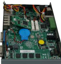
3. Push the Mini PCIe card down and use the provided mounting screws to secure the card on the system board.
