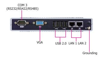
The front panel I/O port consists of the following ports:
