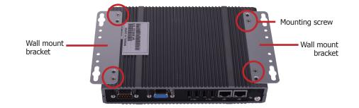
3. The following diagram shows the location and dimension of the wall-mount screw holes.
