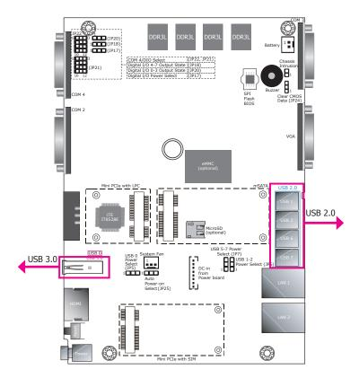
The USB devices allow data exchange between your system and a wide range of simultaneously accessible external Plug and Play peripherals.
