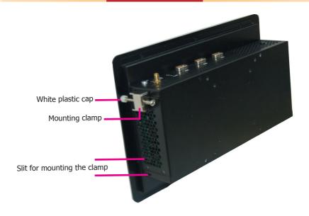
5. The first and second clamps must be positioned and secured diagonally prior to mounting the rest of the clamps. Tighten the clamp's screw using an electric screwdriver by pressing the white plastic cap onto the back of the panel. The illustration below shows that all clamps are properly mounted.
