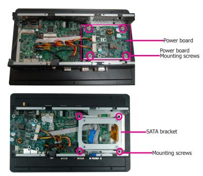
2. Install the SATA drive on the HDD bracket. Place the HDD bracket back to the system and secure the drive in place with the provided mounting screws.
