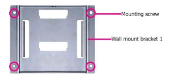
3. Attach the other bracket (Wall mount bracket 2) to the rear of the system.
