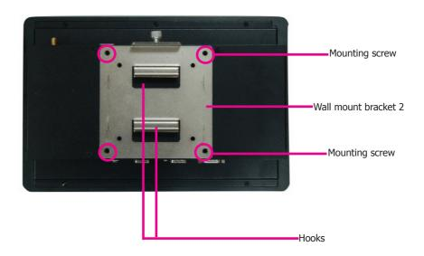
4. Slide the system to "Wall mount bracket 1" to attach the two brackets with the hooks. Then tighten the screw to secure the assembly in place.
