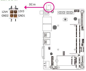
This 4-pin right angle connector is considered a low power solution. Connect a DC power cord to this connector. Using a voltage more than the recommended range may fail to boot the system or cause damage to the system board.
