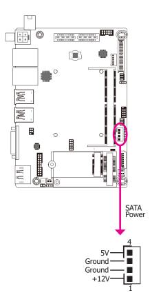
The SATA power connector supplies power to the SATA drive. Connect one end of the provided power cable to the SATA power connector and the other end to your storage device.
