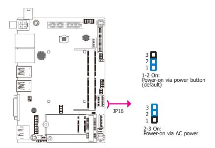
JP16 is used to select the method of powering on the system. If you want the system to power-on whenever AC power comes in, set JP16 pins 2 and 3 to On. If you want to use the power button, set pins 1 and 2 to On.
