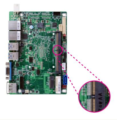
Grasping the module by its edges, align the module into the socket at an approximately 30 degrees angle. Apply firm even pressure to each end of the module until it slips down into the socket. The contact fingers on the edge of the module will almost completely disappear inside the socket.
