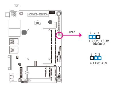
JP12 is used to select the power level of backlight brightness control: +3.3V or +5V.
