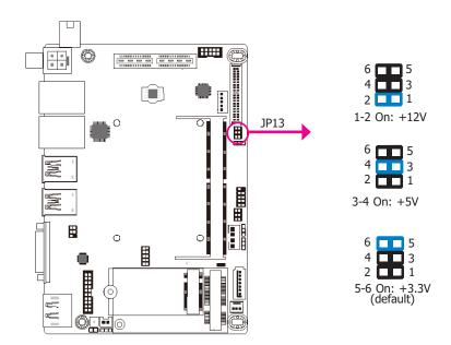
JP13 is used to select the power supplied with the LCD panel.
