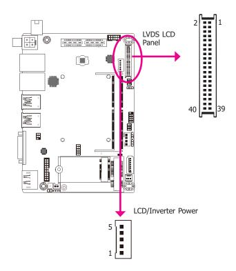
The system board allows you to connect a LCD Display Panel by means of the LVDS LCD panel connector and the LCD/Inverter power connector. These connectors transmit video signals and power from the system board to the LCD panel.
