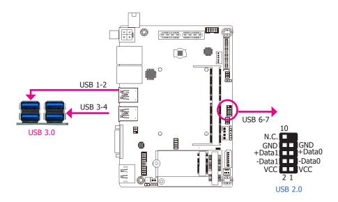
The USB device allows data exchange between your computer and a wide range of simultaneously accessible external plug and play peripherals.
