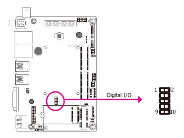
The 8-bit Digital I/O connector provides monitoring and control functions to the connected external devices.
