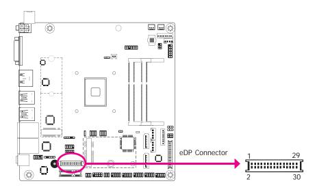
The eDP connector is an embedded displayport which has advanced power-saving features to connect a display device to transmit digital communication of audio and video signals. The table on the right indicates the pin fuctions of the eDP connector.
