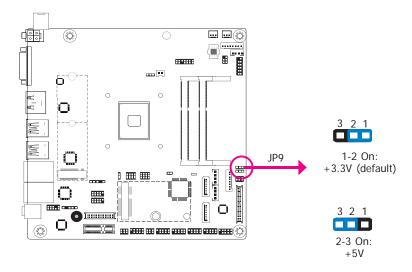
JP9 is used to select the power level of backlight brightness control: +3.3V or +5V.
