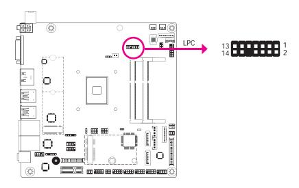
The LPC connector is used for the debug function and its pin functions are listed below.
