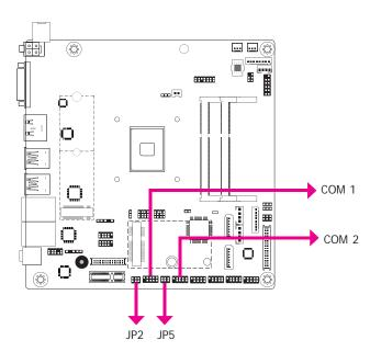
JP2 (for COM 1) and JP5 (for COM 2) are used to configure Serial COM ports to pure RS232 or RS232 with power. The pin functions of COM 1 and COM 2 will vary according to JP2's and JP5's setting respectively.
