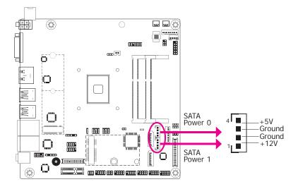
The SATA power connectors supply power to the SATA drive. Connect one end of the provided power cable to the SATA power connector and the other end to your storage device.
