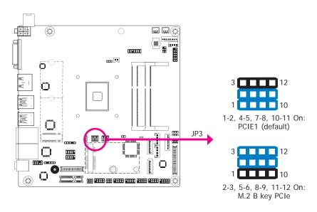
JP3 is used to select the PCIE1 (default) or M.2 B key PCIe signal.
