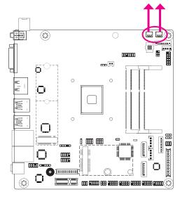
The fan connectors are used to connect cooling fans. The cooling fans will provide adequate airflow throughout the chassis to prevent overheating the CPU and system board components.
