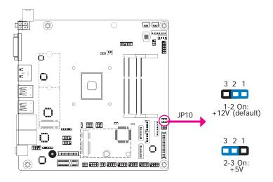
JP10 is used to select the power level of LVDS LCD inverter connector.
