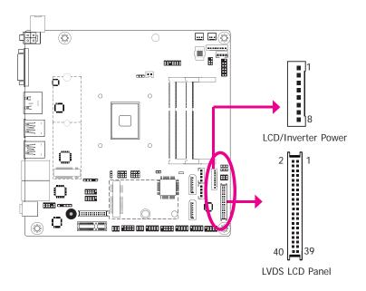
The system board allows you to connect a LCD Display Panel by means of the LVDS LCD panel connectors and the LCD/Inverter power connectors. These connectors transmit video signals and power from the system board to the LCD Display Panel.
