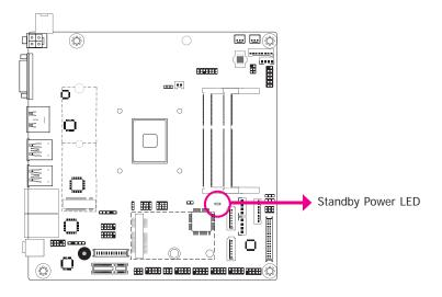
This LED will lit red when the system is in the standby mode. It indicates that there is power on the system board. Power-off the PC and then unplug the power cord prior to installing any devices. Failure to do so will cause severe damage to the motherboard and components.
