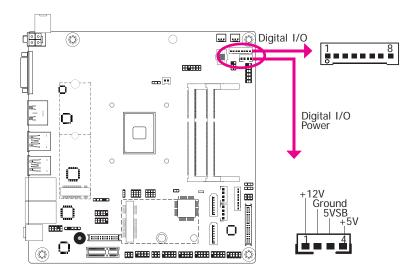
The 8-bit Digital I/O connector provides powering-on function to external devices that are connected to these connectors. The pin functions of the 8-bit digital I/O connector are listed below.
