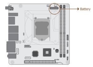
The lithium ion battery addendum supplies power to the real-time clock and CMOS memory as an auxiliary source of power when the main power is shut off.
