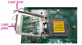
6. Remove the protective cap from the CPU socket. The cap is used to protect the CPU socket against dust and harmful particles. Remove the protective cap only when you are about to install the CPU.
