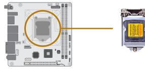
3. Locate the LGA 1151 CPU socket on the system board.
