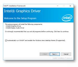
By default, the "Automatically run WinSAT and enable the Windows Aero desktop theme" is enabled. With this enabled, after installing the graphics driver and the system rebooted, the screen will turn blank for 1 to 2 minutes (while WinSAT is running) before the Windows 10 desktop appears. The "blank screen" period is the time Windows is testing the graphics performance.
