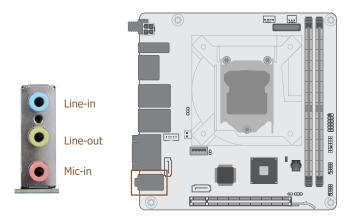
The system board is equipped a rear stacked audio jacks.
