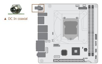
Connect a coaxial DC power cord to the rear coaxial connector for DC supply. Using a voltage higher than the recommended range may result in failure in starting and booting the system
