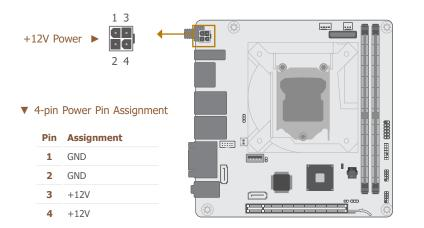
Use a power supply that complies with the ATX12V Power Supply Design Guide Version 1.1. The 4-pin  $\pm$ 12V power connector enables the delivery of more  $\pm$ 12VDC current to the procession
