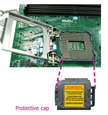
7-1.Insert the CPU into the socket. The gold triangular mark on the CPU must align with the chamfer corner of the CPU socket shown in the photo.
