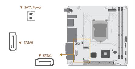
The Serial ATA (SATA) connectors are used to connect the Serial ATA device. SATA 3.0 is supported by the five SATA ports and provides data rate up to 6Gb/s. Connect one end of the Serial ATA cable to a SATA connector and the other end to your Serial ATA device. SATA1, in addition, support Disk on Module (DOM) to which power is supplied via Pin 7.
