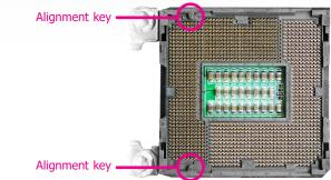
7-3. The CPU's notch will fit into the socket's alignment key when it's seated in the correct orientation.
