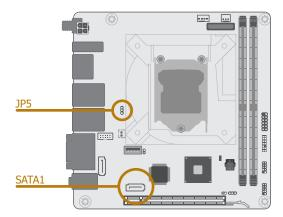
SATA1 supports power supply via power cable or Disk on Module (DOM) to which power is supplied via Pin 7. To switch between the power supply mode, please configure the jumper settings as illustrated below.
