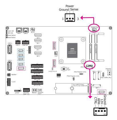
The fan connector is used to connect cooling fan. The cooling fan will provide adequate airflow throughout the chassis to prevent overheating the CPU and system board components.
