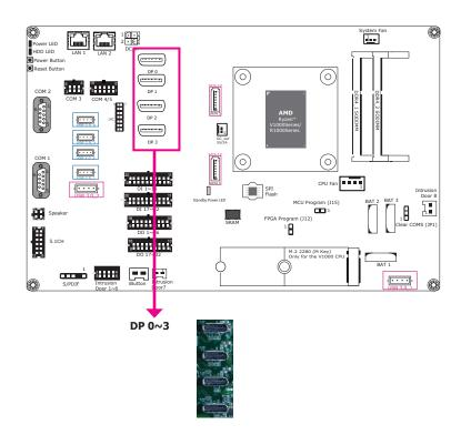
The DisplayPort, a digital display interface, is provided by the integrated AMD® Radeon™ Vega graphics and can be connected to LCD monitors. These ports support resolution up to 4096x2160. Note that the AMD® Ryzen™ V1000 series processors provide 4 DP++ ports whereas the R1000 series processors provide 3 DP++ ports.
