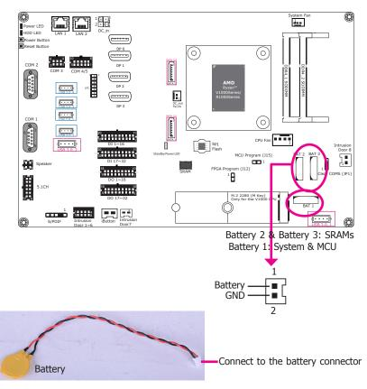
The lithium-ion battery is an auxiliary source of power when the main power is shut off. Two of them provide power for the Static Random-Access Memories (BAT 2 & 3) and one provides power for the MCU and the system's CMOS memory (BAT 1). The batteries for SRAM enables the system to retain data for 5 years without AC power supply. The demonstration application can show the voltage readings as well as set threshold values and its API utility provides functions for battery voltage monitoring.
