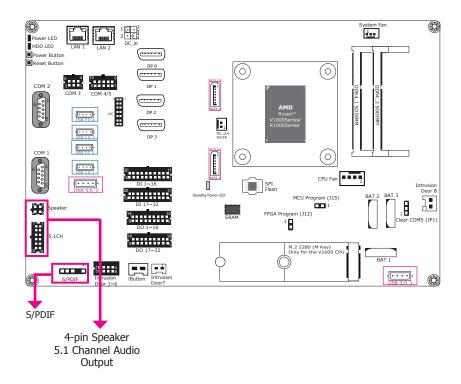
The audio connectors include a 5.1CH audio and a stereo (10W + 10W) speaker output, as well as the digital audio with the S/PDIF connector. These audio ports are provided by Realtek RTL8119 Ethernet Controller and ALC888S High Definiton Audio Codec.
