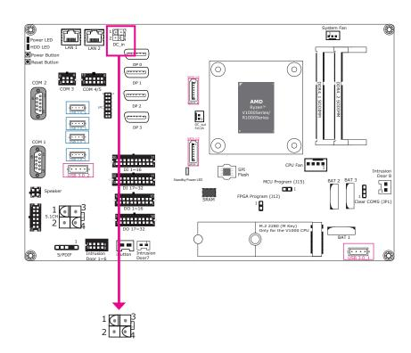
The 4-pin vertical DC-in connector provides a low power input solution. Please use a power adapter with 12V DC output voltage. Using an adapter not compliant to this specification may fail to boot the system or cause damage to the system board.
