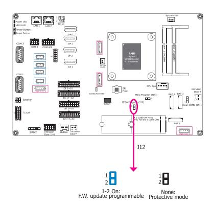
J12 is used to select the FPGA programming mode. To enable or disable FPGA programming of the system board, please set the jumper as indicated above.
