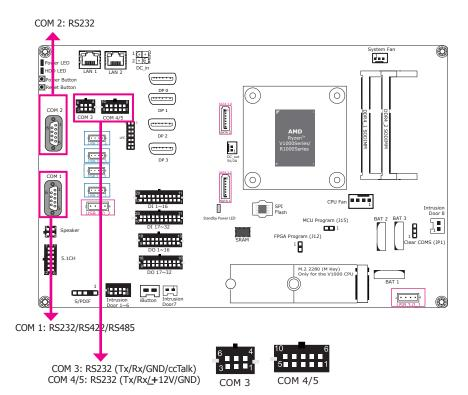
COM 1 and COM 3 can be selected among different communication mode whereas COM 2 can be used in RS232 mode only. COM 3 and COM 4/5 are pin headers and provide signals that are different from typical RS232 communication.
