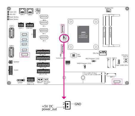
The 2-pin connector provides low power output of 5V/2A.
