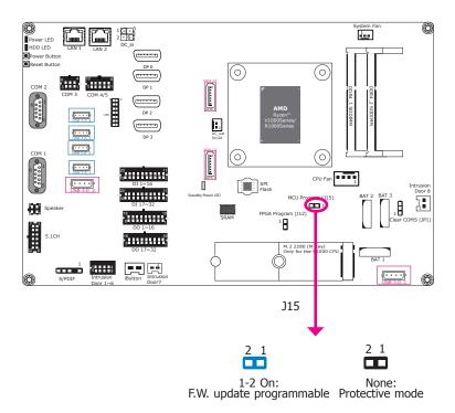
${\sf J15}$  is used to select the MCU programming mode. To enable or disable MCU programming of the system board, please set the jumper as indicated above.
