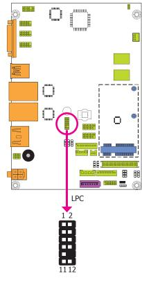
Pin Assignment Pin Assignment Pins Pins CLK 2 LAD1 1 3 RST# 4 LAD0 5 FRAME# 6 VCC\_+3V LAD3 GND 7 8 LAD2 9 10 Х SERIRQ 48MHz 11 12
