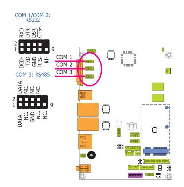
COM 1 and COM 2 are fixed at RS232. COM 3 is fixed at RS485.
