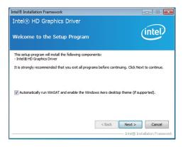
By default, the "Automatically run WinSAT and enable the Windows Aero desktop theme" is enabled. With this enabled, after installing the graphics driver and the system rebooted, the screen will turn blank for 1 to 2 minutes (while WinSAT is running) before the Windows 7/ Windows 8 desktop appears. The "blank screen" period is the time Windows is testing the graphics performance.
