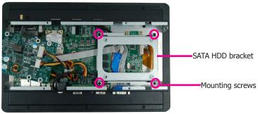
Align the mounting holes of the SATA drive with the mounting holes on the SATA HDD bracket and use the provided mounting screws to attach the SATA drive to the bracket.
