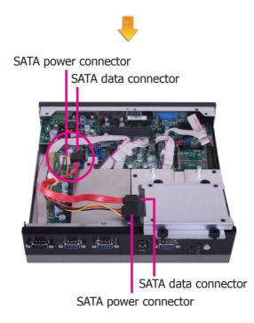
5. Place the SATA drive with the HDD bracket into the system. Align the mounting holes on the HDD bracket with the mounting holes on the protective plate and then use the provided mounting screws to secure the drive in place.
