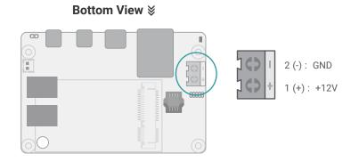
This 2-pin terminal block is considered a low power solution. Connect a DC power cord to this terminal block by inserting the wire into the block and then screw tight the screw on top to secure the wire in place. Please make sure the positive and negative wires are installed correctly. Using a voltage more than the recommended range may fail to boot the system or cause damage to the system board.
