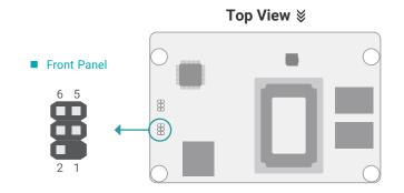
The SMBus (System Management Bus) connector is used to connect the SMBus device. It is a multiple device bus that allows multiple chips to connect to the same bus and enable each one to act as a master by initiating data transfer.
