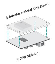
The heat spreader is designed to be mounted onto the module as illustrated below. Please make sure the contacting sides of the heat spreader and the module are correct - the CPU side of the module shall be facing the interface metal side and legs of the heat spreader. Rotate horozontally so the interface metal sits right on top of the CPU. Remove any plastic cover on the interface metal and apply thermal paste/adhesive if it is required.
