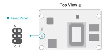
The **Pin 1** of Front Panel cable should be connected to Front Panel **Pin 6** on the motherboard. Due to Pin definition on GHF51 different from other boards, the HDD\_LED (Red) doesn't function.
