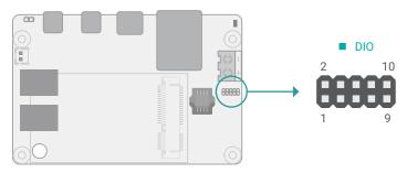
The 8-bit Digital I/O (DIO) connector allows for input/output signals of digital logical states defined by voltage levels.
