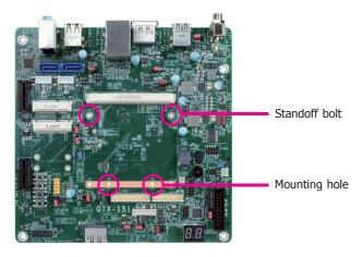
2. Grasping AL700 by its edges, insert it into the carrier board, and you will hear a distinctive "click" indicating AL700 is correctly locked into position.
