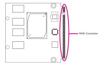
The MXM connector is used to interface with the carrier board. Insert AL700 to the MXM connector on the carrier board. Refer to the following pages for the pin functions of this connector.
