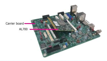
3. Press down AL700 and put on the heat sink on top of AL700 with its mounting holes and bolts aligned on the carrier board. Use the mounting screws to fix AL700 and heat sink in place.
