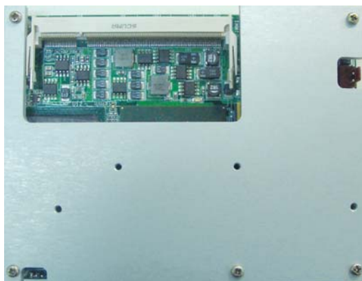
Heatspreader on G5C900-B (top view)
