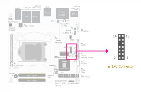
The LPC connector is used for debugging and its pin functions are listed below.
