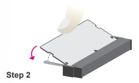
Press the end of the card far from the socket down while making sure the retention notch and the clip align as indicated by the dotted line in the illustration. If the retention notch and the clip do not align, please remove the card and re-insert it. Press the card all the way down.
