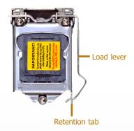
5. Lift the load lever and the load plate all the way up as shown in the photo.
