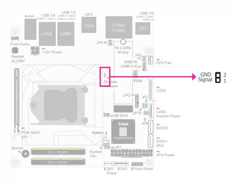
The board supports the chassis intrusion detection function. Connect the chassis intrusion sensor cable from the chassis to this connector. When the system's power is on and a chassis intrusion occurred, an alarm will sound. When the system's power is off and a chassis intrusion occurred, the alarm will sound only when the system restarts.
