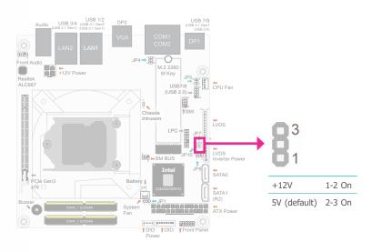
JP10 is used to select the power level of LVDS Inverter: +5V (default) or +12V.
