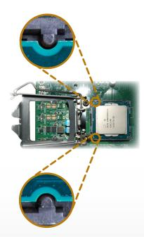
8. Close the load plate then push the load lever down.
