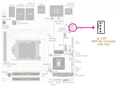
The fan connector is used to power a cooling fan. Cooling fans will provide adequate airflow throughout the chassis to prevent overheating the CPU and system board components. The 4-pin fans provide PWM to modulate fan speed.
