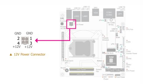
Connect a ATX 4-pin power to this jack.
