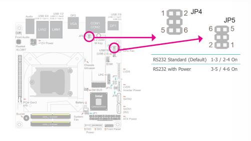
JP4 (for COM 1) and JP5 (for COM 2) are designed to configure Serial COM ports to pure RS232 or RS232 with power.
