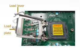
Remove the protective cap from the CPU socket. The cap is used to protect the CPU socket against dust and harmful particles. Remove the protective cap only when you are about to install the CPU.
