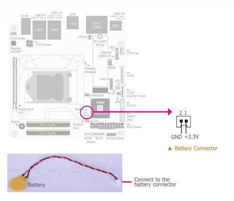
The lithium ion battery addendum supplies power to the real-time clock and CMOS memory as an auxiliary source of power when the main power is shut off.
