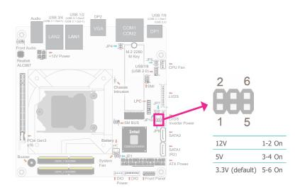
JP8 is used to select the power supplied with the LVDS LCD panel.
