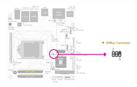
The SMBus (System Management Bus) connector is used to connect the SMBus device. It is a multiple device bus that allows multiple chips to connect to the same bus and enable each one to act as a master by initiating data transfer.
