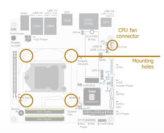
Screw tight two of the spring screws at opposite corners into the mounting holes. And then proceed with the other two spring screws.
