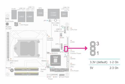
JP7 is used to select the power level of backlight control: +3.3V (default) or +5V.
