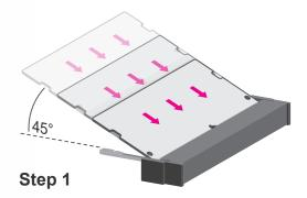
Insert the memory card into the slot while making sure 1) the notch and the key are aligned, and 2) the non-connector end rises approximately 45 degrees horizontally. Press the card firmly into the socket while applying and maintaining even pressure on both ends.
