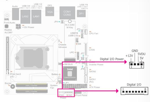
The 8-bit Digital I/O connector provides powering-on function to external devices that are connected to these connectors.
