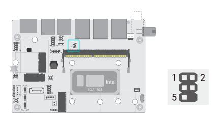
The SMBus (System Management Bus) connector is used to connect the SMBus device. It is a multiple device bus that allows multiple chips to connect to the same bus and enable each one to act as a master by initiating data transfer.
