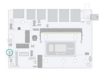
DPJP604 is used to select the panel backlight power.
