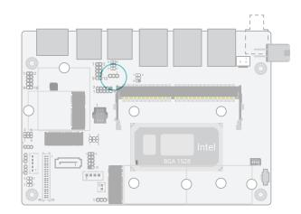
JP2 is used to select the power of DIO (Digital I/O) signal.
