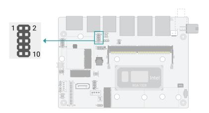
The Front Audio internal connector allows you to connect to the second line-out and mic-in jacks that are at the front panel of your system.
