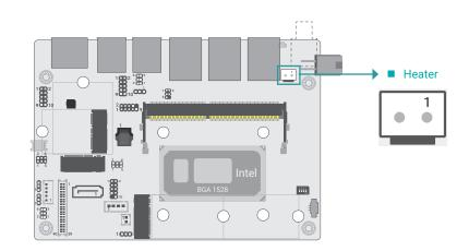
The heater box header provides 12V power to the external heater with a 2-pin pin header for On/Off switch.
