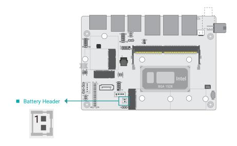
The lithium ion battery powers the real-time clock and CMOS memory. It is an auxiliary source of power when the main power is shut off.
