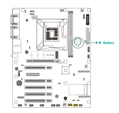
The lithium ion battery addendum supplies power to the real-time clock and CMOS memory as an auxiliary source of power when the main power is shut off. Insert a coin cell battery into the holder and make sure the polarities are correctly oriented – the cap side (rimmed rounded edge) is negative and should be facing the holder; the flat side with a + mark is positive and should be facing away from the holder.
