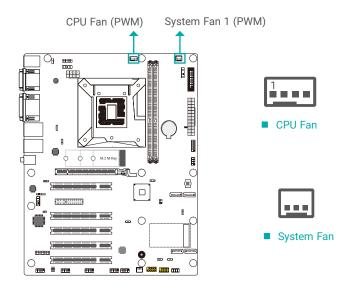
These fan connectors are used to connect cooling fans. The cooling fans will provide adequate airflow throughout the chassis to prevent overheating the CPU and system board components.
