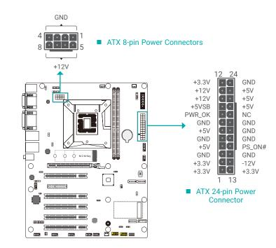
Use a power supply that complies with the ATX12V Power Supply Design Guide Version 1.1. An ATX12V power supply unit has a standard 24-pin ATX main power connector that must be inserted into the 24-pin connector. The 8-pin +12V power connector enables the delivery of more +12VDC current to the processor's Voltage Regulator Module (VRM).
