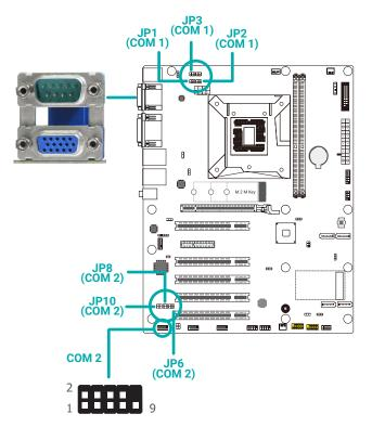
JP1/JP2/JP3 (for COM 1) and JP6/JP8/JP10 (for COM 2) are used to configure the COM ports to RS232, RS422 (Full Duplex) or RS485. When COM 1 RS232/422/485 is selected, JP1 and JP2 must be set in accordance to JP3. When COM 2 RS232/422/485 is selected, JP6 and JP8 must be set in accordance to JP10. The pin functions of the COM ports will vary according to the jumpers' setting.
