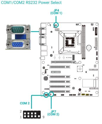
JP4 (for COM 1) and JP7 (for COM 2) are used to configure Serial COM ports to pure RS232 or RS232 with power. The pin functions of COM 1 and COM 2 will vary according to JP4's and JP7's setting respectively.
