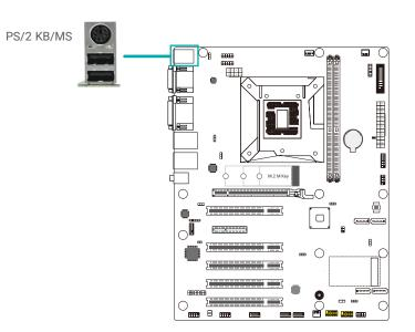
This rear I/O port is used to connect a PS/2 mouse and a PS/2 keyboard. The PS/2 mouse port uses mini-DIN-6.
