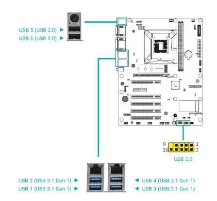
The USB device allows data exchange between your computer and a wide range of simultaneously accessible external Plug and Play peripherals. The system board is equipped with multiple USB ports as listed below:
