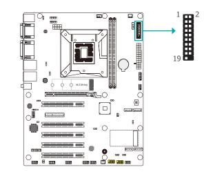
The 8-bit Digital I/O connector provides powering-on function to external devices that are connected to these connectors. The pin functions of the 8-bit digital I/O connector are listed below.
