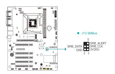
The SMBus (System Management Bus) connector is used to connect SMBus devices. It is a multiple device bus that allows multiple chips to connect to the same bus and enable each one to act as a master by initiating data transfer.
