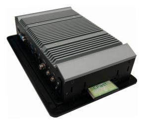
2. Close the CFast card cover and attach the screw. To eject the card, push the card inward to release the lock and pull it out.
