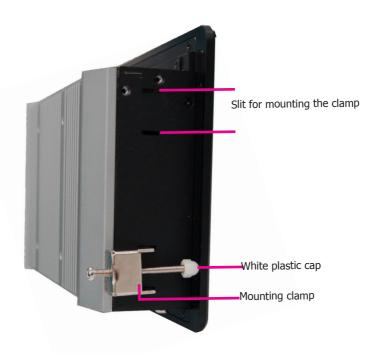
6. The first and second clamps must be positioned and secured diagonally prior to mounting the rest of the clamps. Tighten the clamp's screw using an electric screwdriver by pressing the white plastic cap onto the back of the panel. The illustration below shows that all clamps are properly mounted.
