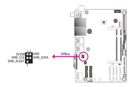
The SMBus (System Management Bus) connector is used to connect SMBus devices. It is a multiple device bus that allows multiple chips to connect to the same bus and enable each one to act as a master by initiating data transfer.
