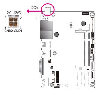
The 4-pin right-angle connector on the system board co-lays with a DC-in jack (optional) or 4-pin vertical type connector (optional) as the photo displayed below.
