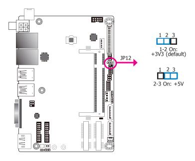
JP12 is used to select the power level of backlight brightness control: +3.3V or +5V.
