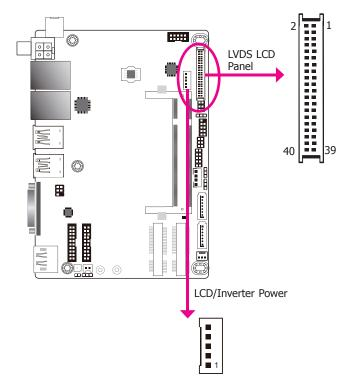
The system board allows you to connect a LCD Display Panel by means of the LVDS LCD panel connector and the LCD/Inverter power connector. These connectors transmit video signals and power from the system board to the LCD panel.
