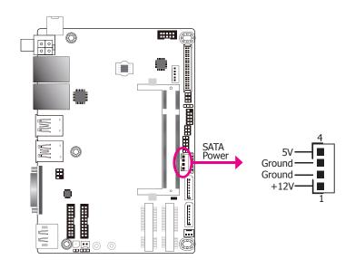
The SATA power connector supplies power to the SATA drive. Connect one end of the provided power cable to the SATA power connector and the other end to your storage device.
