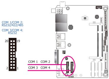
COM 1 and COM 2 can be selected among RS232, RS422 and RS485. COM 3 and COM 4 are fixed at RS232. Configure COM 1 and COM 2 serial communication mode in the BIOS ("SIO NUVOTON6106D" submenu of the Advanced menu).
