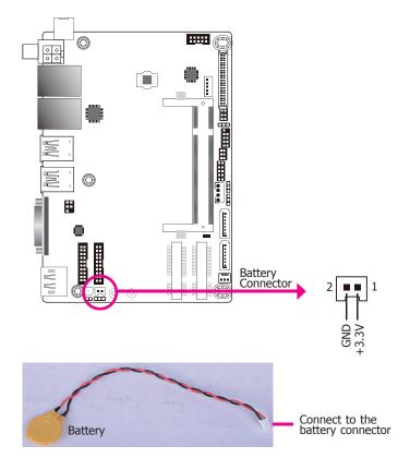
The lithium ion battery powers the real-time clock and CMOS memory. It is an auxiliary source of power when the main power is shut off.
