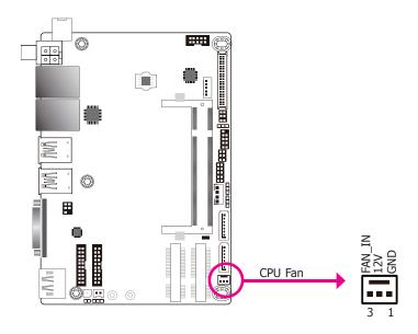
The fan connector is used to connect the cooling fan. The cooling fan will provide adequate airflow throughout the chassis to prevent overheating the CPU and system board components.
