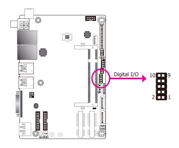
The 8-bit Digital I/O connector provides monitoring and control functions to the connected external devices.
