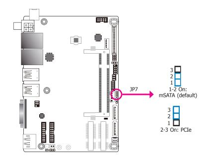
JP7 is used to select the Mini PCIe slot (full-size) signal: PCIe or mSATA (default).
