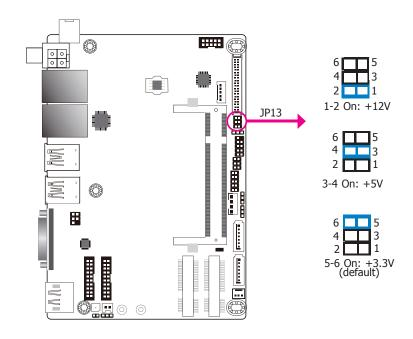
JP13 is used to select the power supplied with the LCD panel.
