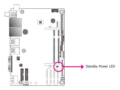
This LED will lit red when the system is in the standby mode. It indicates that there is power on the system board. Power-off the PC and then unplug the power cord prior to installing any devices. Failure to do so will cause severe damage to the motherboard and components.
