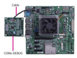
Use the long mounting screws to secure the heat sink on the top of the BT968 and the COMe-LINK1 debug card and connect the cooling fan's cable to the fan connector on BT968. The photo below shows the locations of long mounting screws.
