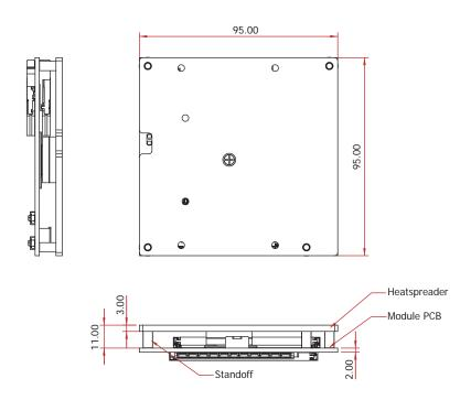
Side View of the Module with Heat Sink and Carrier Board
