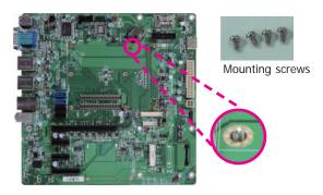
3. While supporting the mounting screw at the bottom, from the top side of the board, fasten a bolt into the screw.
