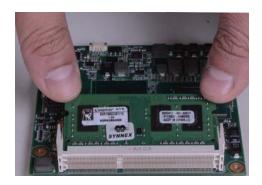
6. Push down the module until the clips at each end of the socket lock into position. You will hear a distinctive "click", indicating the module is correctly locked into position.
