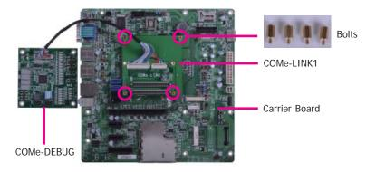
5. Grasp BT968 by its edges to press it down on the top of the COMe-LINK1 debug card.
