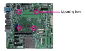
2. Insert the provided mounting screws into the mounting holes - from the bottom through the top of the carrier board.
