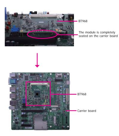
9. Use the provided mounting screws to secure BT968 with heat sink to the carrier board and then connect the cooling fan's cable to the fan connector on BT968. The photo below shows the locations of the long mounting screws.
