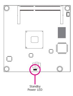
This LED will light when the system is in the standby mode.
