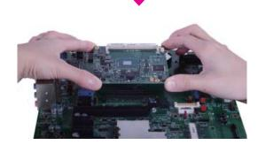
7. Press BT968 down firmly until it is completely seated on the COM Express connectors of the carrier board.
