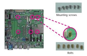
4. Use the provided bolts to fix the COMe-LINK1 debug card onto the carrier board.
