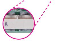
Grasping the module by its edges, align the module into the socket at an approximately 30 degrees angle. Apply firm even pressure to each end of the module until it slips down into the socket. The contact fingers on the edge of the module will almost completely disappear inside the socket.
