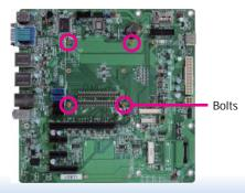
6. Grasping BT968 by its edges, position it on top of the carrier board with its mounting holes aligned with the bolts on the carrier board. This will also align the COM Express connectors of the two boards to each other.
