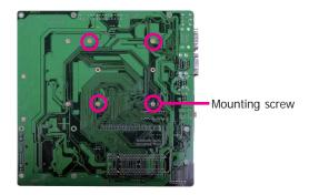
5. The photo below shows the component side of the board with the bolts already fixed in place.
