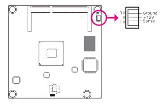
Connect the CPU fan's cable connector to the CPU fan connector on the board. The cooling fan will provide adequate airflow throughout the chassis to prevent overheating the CPU and board components.
