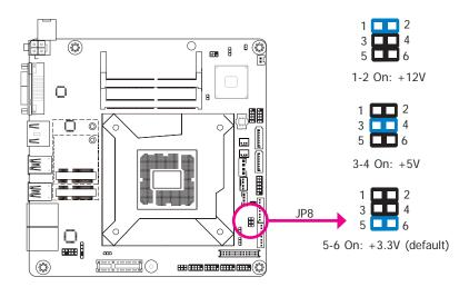
JP8 is used to select the power supplied with the LCD panel.
