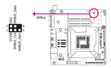
The SMBus (System Management Bus) connector is used to connect SMBus devices. It is a multiple device bus that allows multiple chips to connect to the same bus and enable each one to act as a master by initiating data transfer.
