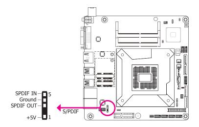
The S/PDIF connector is used to connect an external S/PDIF port. Your S/PDIF port may be mounted on a card-edge bracket. Install the card-edge bracket to an available slot at the rear of the system chassis then connect the audio cable to the S/PDIF connector. Make sure pin 1 of the audio cable is aligned with pin 1 of the S/PDIF connector.
