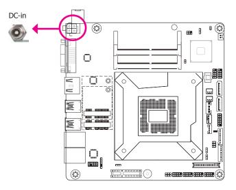
This jack is considered a low power solution. Connect a DC power cord to this jack. Using a voltage more than the recommended range may fail to boot the system or cause damage to the system board.
