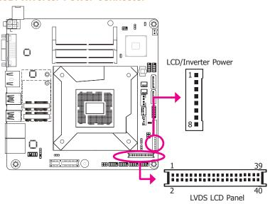
The system board allows you to connect a LCD Display Panel by means of the LVDS LCD panel connector and the LCD/Inverter power connector. These connectors transmit video signals and power from the system board to the LCD Display Panel.
