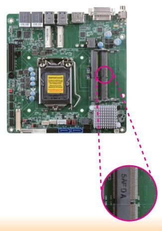
Grasping the module by its edges, align the module into the socket at an approximately 30 degrees angle. Apply firm even pressure to each end of the module until it slips down into the socket. The contact fingers on the edge of the module will almost completely disappear inside the socket.
