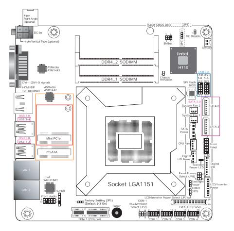
SD101-H110: 12V DC-in jack (default) or 4-pin power Right/Vertical Angle Connector (optional).
