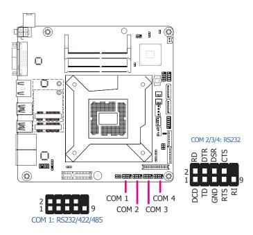
The pin functions of COM 1 will vary according to BIOS' setting. JP2 (for COM1) is designed to configure Serial COM port to pure RS232 or RS232 with power. Refer to "COM 1 RS232/Power Select" in this chapter for more information.
