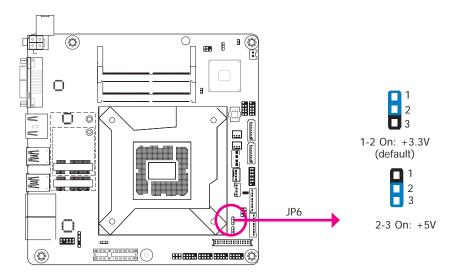
JP6 is used to select the power level of backlight brightness control: +3.3V or +5V.
