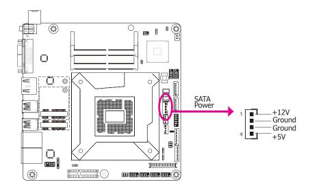
This SATA power connector supplies power to the SATA drive. Connect one end of the provided power cable to the SATA power connector and the other end to your storage device.
