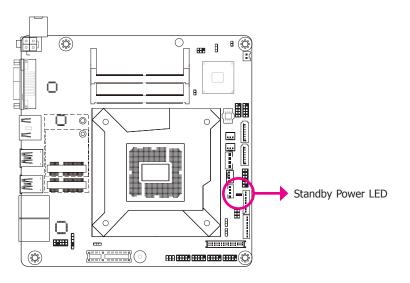
This LED will light red when the system is in the standby mode. It indicates that there is power on the system board. Power-off the PC and then unplug the power cord prior to installing any devices. Failure to do so will cause severe damage to the motherboard and components.
