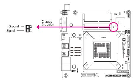
The board supports the chassis intrusion detection function. Connect the chassis intrusion sensor cable from the chassis to this connector. When the system's power is on and a chassis intrusion occurred, an alarm will sound. When the system's power is off and a chassis intrusion occurred, the alarm will sound only when the system restarts.
