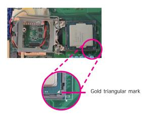
The CPU's notch will at the same time fit into the socket's alignment key.
