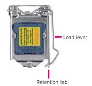
Lifting the load lever will at the same time lift the load plate.
