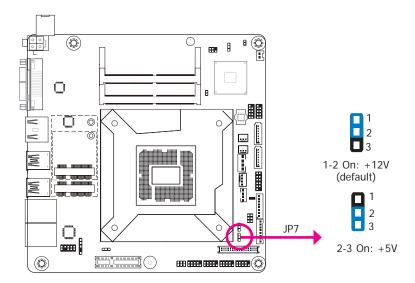
JP7 is used to select the power level of the LVDS LCD/inverter power connector.
