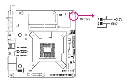
The lithium ion battery powers the real-time clock and CMOS memory. It is an auxiliary source of power when the main power is shut off.
