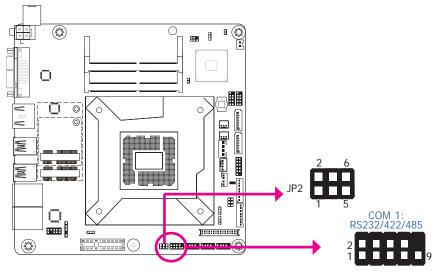
JP2 (for COM 1) is designed to configure the Serial COM port to pure RS232 or RS232 with power. The pin functions of COM 1 will vary according to JP2's setting respectively.
