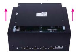
5. The SODIMM socket and the Mini PCie slot are readily accessible after removing the chassis cover.
