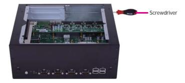
4. Insert one expansion card with a bracket into the PCI slot and the PCIe x16 slot respectively that are on the riser card and secure the bracket in place.
