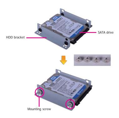
3. Place the SATA drive (with HDD brackets) into the system. Align the mounting holes on the HDD brackets with the mounting holes on the heat-dissipating plate and then use the provided mounting screws to secure the drive in place.
