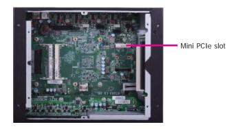
2. The system board is equipped with 1 Mini PCIe slot. The Mini PCIe slot supports a half length or a full length Mini PCIe card. Note the key on the slot. The key ensures the Mini PCIe card can be plugged into the slot in one direction only.
