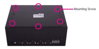
4. After removing the mounting screws, lift the cover up.
