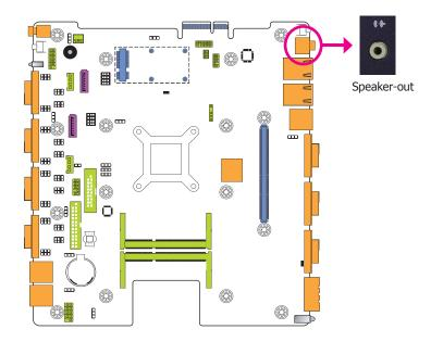
This speaker-out jack is used to connect a headphone or external speakers.
