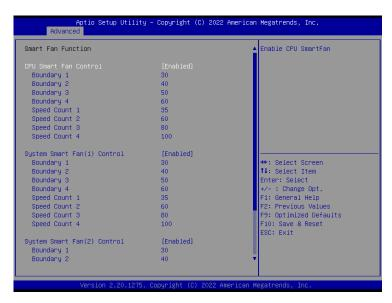
Smart Fan is a fan speed moderation strategy dependent on the current system temperature. When the system temperature goes higher than the Boundary setting, the fan speed will be turned up to the setting of the Fan Speed Count that bears the same index as the Boundary field.
