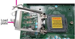
6. Remove the protective cap from the CPU socket. The cap is used to protect the CPU socket against dust and harmful particles. Remove the protective cap only when you are about to install the CPU.
