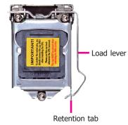
The CPU socket must not come in contact with anything other than the CPU. Avoid unnecessary exposure. Remove the protective cap only when you are about to install
