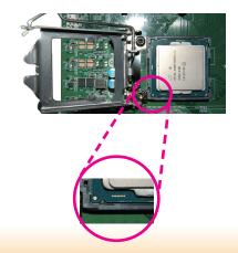
8. Close the load plate then push the load lever down.
