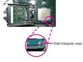
The CPU's notch will prop-erly fit into the socket's alignment key.
