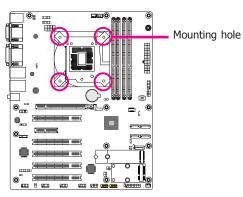
Orient the heat sink such that the CPU fan's cable is nearest the CPU fan connector.
