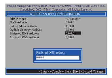
35. Select **Alternate DNS Address** then press Enter. Enter address then press Enter.
