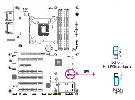
JP9 is designed to select the Mini PCIe signal: mSATA or Mini PCIe (default).
