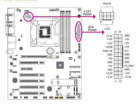
Use a power supply that complies with the ATX12V Power Supply Design Guide Version 1.1. An ATX12V power supply unit has a standard 24-pin ATX main power connector that must be inserted into the 24-pin connector. The 8-pin  $\pm$ 12V power connector enables the delivery of more  $\pm$ 12VDC current to the processor's Voltage Regulator Module (VRM).
