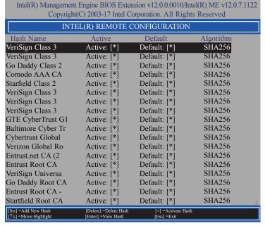
47. Press Esc until you return to the Intel(R) AMT Configuration menu, select Power Control then press Enter. In the Intel(R) AMT Power Control menu, select Intel(R) AMT ON in Host Sleep States then press Enter. Select an option then press Enter.
