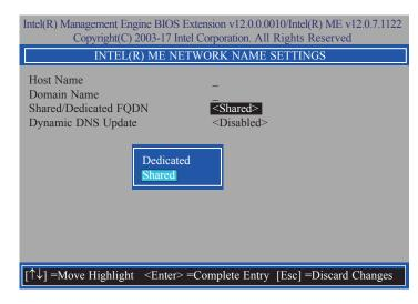
Select Dynamic DNS Update then press Enter. Select Enabled or Disabled then press Enter. If Dynamic DNS Update is set to Enabled, Periodic Update Interval and TTL fields will show up.
