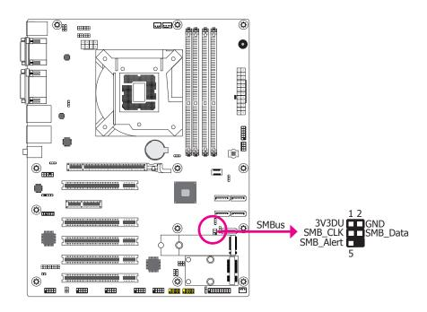
The SMBus (System Management Bus) connector is used to connect SMBus devices. It is a multiple device bus that allows multiple chips to connect to the same bus and enable each one to act as a master by initiating data transfer.
