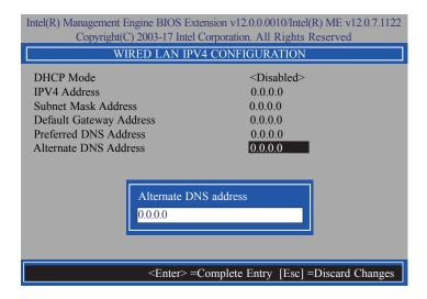
Press Esc until you return to the Intel(R) AMT Configuration menu. If you want to activate the current network settings and open the ME network inferface, select Activate Network Access, press Enter, then press Y.
