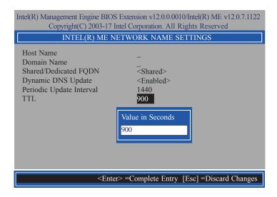
Press Esc until you return to the Intel(R) ME Network Setup menu. Select TCP/IP Settings then press Enter. In the TCP/IP Settings menu, select Wired LAN IPV4 Configuration then press Enter.
