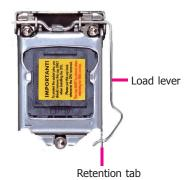
5. Lift the load lever to lift the load plate.
