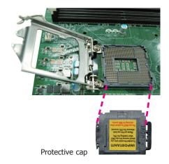
7. Insert the CPU into the socket. The gold triangular mark on the CPU must align with the corner of the CPU socket shown on the photo.
