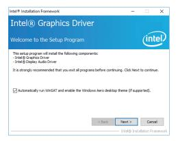
By default, the "Automatically run WinSAT and enable the Windows Aero desktop theme" is enabled. With this enabled, after installing the graphics driver and the system rebooted, the screen will turn blank for 1 to 2 minutes (while WinSAT is running) before the Windows 10 desktop appears. The "blank screen" period is the time Windows is testing the graphics performance.
