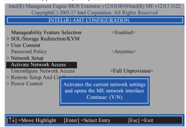
In the Intel(R) AMT Configuration menu, select Unconfigure Network Access then press Enter.
