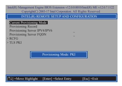
In the Intel(R) Remote Setup And Configuration menu, select Provisioning Record then press Enter.
