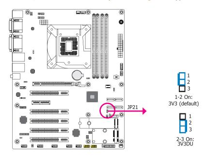
JP21 is designed to select the Mini PCIe/mSATA power: 3V3 (default) or 3V3DU.
