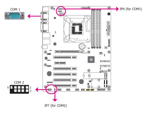
JP4 (for COM 1) and JP7 (for COM 2) are used to configure Serial COM ports to pure RS232 or RS232 with power. The pin functions of COM 1 and COM 2 will vary according to JP4's and JP7's settings respectively.
