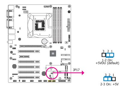
JP17 is used to select the power of DIO (Digital I/O) signal: +5VDU (default) or +5V.
