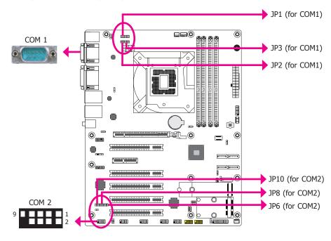
JP1/JP2/JP3 (for COM1) and JP6/JP8/JP10 (for COM2) are used to configure the COM ports to RS232, RS422 (Full Duplex) or RS485. When COM 1 RS232/422/485 is selected, JP2 and JP3 must be set in accordance to JP1. When COM 2 RS232/422/485 is selected, JP6 and JP8 must be set in accordance to JP10. The pin functions of the COM ports will vary according to the jumpers' setting.
