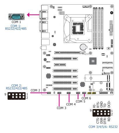
The pin functions of COM 1 port will vary according to setting of JP1, JP2, JP3 and JP4. Refer to "COM1/COM2 RS232/422/485 Select" and "COM1/COM2 RS232/Power Select" in this chapter for more information.
