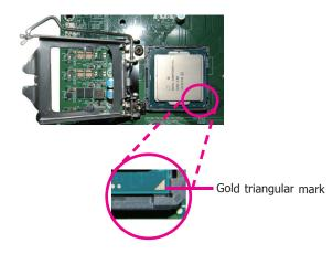
The CPU's notch will properly fit into the socket's alignment key.
