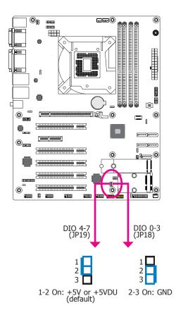
Based on the power level of DIO (Digital I/O) selected on JP17, JP18 (DIO pin 0-3) and JP19 (DIO pin 4-7) are used to select the output state of Digital I/O: pull high or pull low. When selecting pull high, the power selection will be the same as the JP17's setting.
