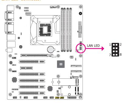
The LAN LED connector is used to detect the connection state of RJ45 LAN ports when the connection is made to an active network via a cable. The pin functions of the LAN LED connector are listed below.
