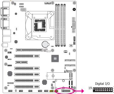
The 8-bit Digital I/O connector provides powering-on function to external devices that are connected to these connectors.
