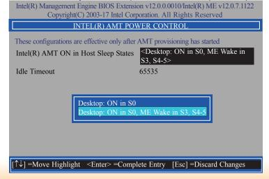
48. In the **Intel(R) AMT Power Control** menu, select **Idle Timeout** then press Enter. Enter the timeout value and press Enter.
