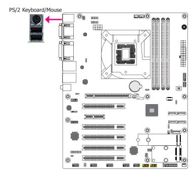
This rear I/O port is used to connect a PS/2 keyboard/mouse. The PS/2 mouse port uses IRO12.
