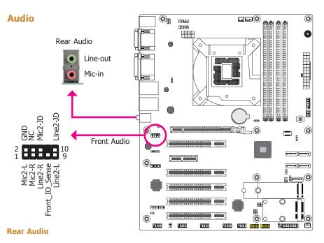
The system board is equipped with 2 audio jacks (Line-out and Mic-in). Line-in jack is available upon request. A jack is a one-hole connecting interface for inserting a plug.
