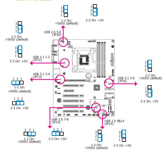
JP12, JP13, JP14, JP15, JP16 and JP20 are used to select the power of the USB ports. Selecting +5VDU will allow you to use a USB device to wake up the system.
