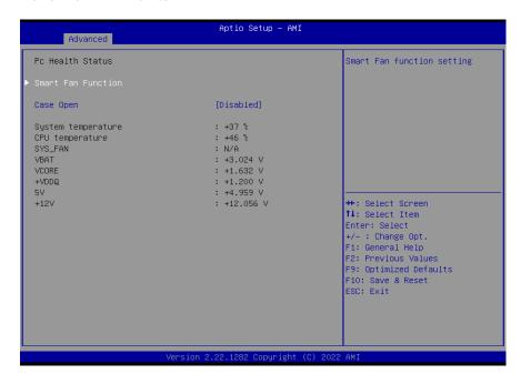
This section displays the system's health information, i.e. voltage readings, CPU and system temperatures, and fan speed readings
