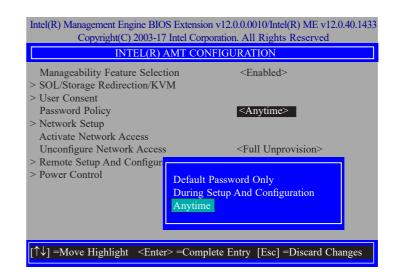
Under the Intel(R) AMT Configuration menu, select Password Policy then press Enter. You may choose to use a password only during setup and configuration or to use a password anytime the system is being accessed.
