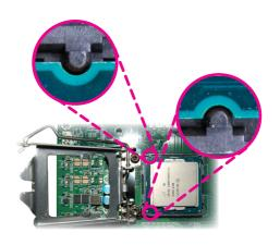
8. Close the load plate then push the load lever down.
