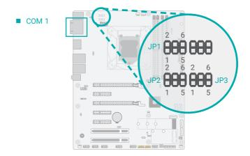
JP1, JP2, and JP3 are used to configure the COM 1 port to RS232, RS422 (Full Duplex) or RS485. The three jumpers must all be configured to the same serial mode.
