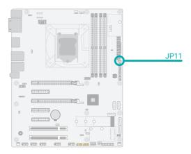
Power of the system can be turned on via the Power Button or via the AC-In signal. Switch the setting by putting the jumper caps on neighboring pins of JP11 as listed and illustrated below:
