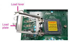
Remove the protective cap from the CPU socket. The cap is used to protect the CPU socket against dust and harmful particles. Remove the protective cap only when you are about to install the CPU.
