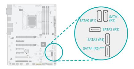
The Serial ATA (SATA) connectors are used to connect the Serial ATA device. SATA 3.0 is supported by the five SATA ports and provides data rate up to 6Gb/s. Connect one end of the Serial ATA cable to a SATA connector and the other end to your Serial ATA device.
