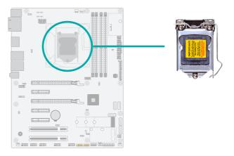
3. Locate the LGA 1151 CPU socket on the system board.
