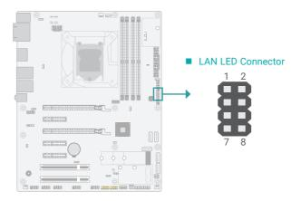
The LAN LED connector is used to detect the connection state of RJ45 LAN ports when the connection is made to an active network via a cable. The pin functions of the LAN LED connector are listed below.
