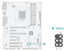
The SMBus (System Management Bus) connector is used to connect the SMBus device. It is a multiple device bus that allows multiple chips to connect to the same bus and enable each one to act as a master by initiating data transfer.
