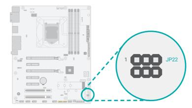
The power of Mini PCle can be switched between 3V3DU and 3V3 via JP22.
