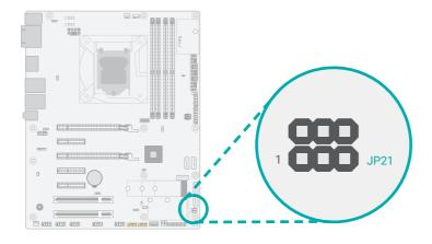
The signal of Mini PCle can be switched between mSATA (default) or PCle via JP21.
