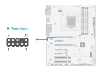
The Front Audio internal connector allows you to connect to the second line-out and mic-in jacks that are at the front panel of your system.
