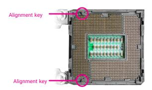
7-3.The CPU's notch will fit into the socket's alignment key when it's seated in the correct orientation.
