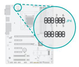
The COM 1 serial port supports RS232 with or without power configured via jumper settings of JP4.
