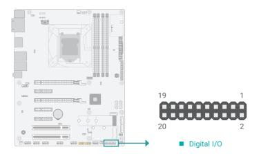
The 8-bit Digital I/O (DIO) connector allows for input/output signals of digital logical states defined by voltage levels.
