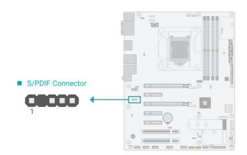
The Sony/Philips Digital Interface (S/PDIF) connector is for audio output to external audio equipment. The S/PDIF port may be mounted on a card-edge bracket. Install the card-edge bracket to an available slot at the rear of the system chassis then connect the audio cable to the S/PDIF connector. Make sure pin 1 of the audio cable is aligned with pin 1 of the S/PDIF connector.
