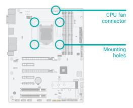
4. Screw tight two of the spring screws at opposite corners into the mounting holes. And then proceed with the other two spring screws.
