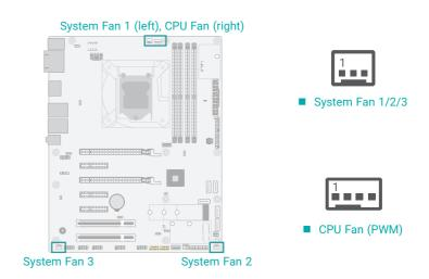
These fan connectors are used to connect to cooling fans. Cooling fans provide adequate air circulation throughout the chassis and dissipate heat to prevent overheating of the system board and components. The 4-pin fan provides PWM to modulate fan speed whereas the 3-pin fans modulate fan speed via voltage modulation.
