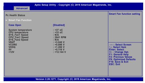
This section displays the system's health information, i.e. voltage readings, CPU and system temperatures, and fan speed readings.
