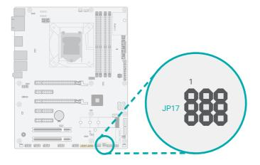
JP17 is used to select the power of Digital I/O: +5VDU (default) or +5V.
