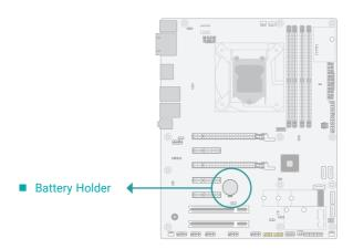
The lithium ion battery addendum supplies power to the real-time clock and CMOS memory as an auxiliary source of power when the main power is shut off. Insert a coin cell battery into the holder and make sure the polarities are correctly oriented — the cap side (rimmed rounded edge) is negative and sould be facing the holder; the flat side with a + mark is positive and should be facing away from the holder.
