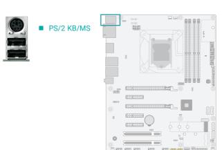
This rear I/O port is used to connect a PS/2 keyboard/mouse. IRQ12 is reserved for the PS/2 mouse connector.
