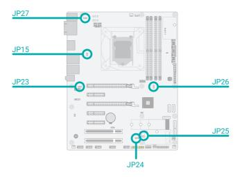
The power of the USB connectors' voltage buses can be configured to either 5VDU or 5V. The jumpers are located as illustrated above and correspond to each USB port number as listed.
