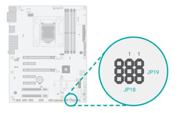
The Digital I/O can be configured to use the power bus of the Digital I/O connector for power supply or not. JP18 is used to select for DIO0~DIO3. JP19 is used to select for DIO4~DIO7.
