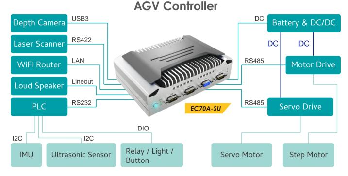
The DFI EC70A-SU/KU series not only bring reliable energy-efficiency, durability, and stability, but also provide a complete I/O interface, ranging from sensors, wireless networks, power supplies, and power systems. It fully meets the need for AMR.
