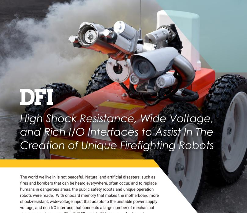
structures and sensors, DFI's SU253 assists Chinese manufacturers to develop a firefighting robot as a substitute for firefighters in dangerous situations at the scene of the accident.
