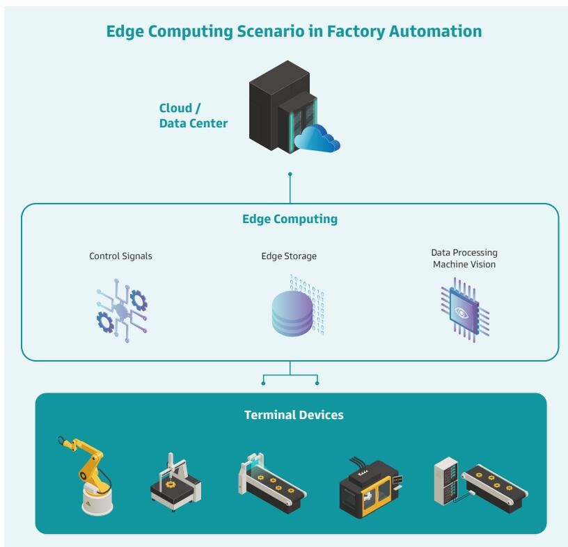
An example architecture for edge computing in factory automation applications. The terminal device communicates with the edge computing server and sends back the data. The server analyzes the data, sends back the corresponding control commands, and stores the data locally and then sends it back to the cloud if necessary. The cloud host should minimize the need for real-time analysis to avoid communication delays.
