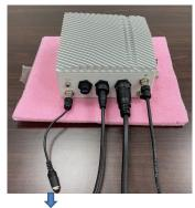
This is a standard power converter cable after assembly; customer can either use our power converter cable or a customized cable to directly connect ECX700 with their power adaptor
