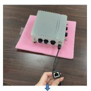
This is a standard LAN converter cable after assembly; customer can either use our converter cable or a customized cable to directly connect ECX700 with their devices
