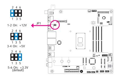
JP1 is used to select the power supplied with the eDP panel.
