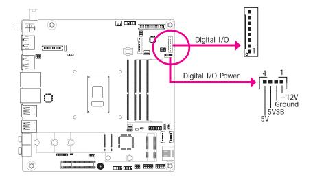
The 8-bit Digital I/O connector provides powering-on function to external devices that are connected to the connector.
