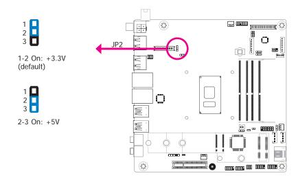
JP2 is used to select the power level of backlight control: +3.3V (default) or +5V.
