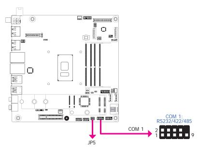
JP5 is designed to configure the Serial COM port 1 to pure RS232 or RS232 with power. The pin functions of COM 1 will vary according to JP5's setting.
