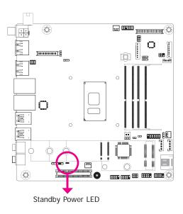
This LED will lit red when the system is in the standby mode. It indicates that there is power on the system board. Power-off the PC and then unplug the power cord prior to installing any devices. Failure to do so will cause severe damage to the motherboard and components.
