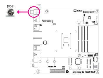
Connect a DC power cord to the DC-in jack. Using a voltage more than the recommended range may fail to boot the system or cause damage to the system board.
