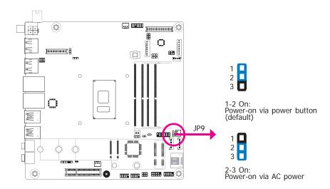
JP9 is used to select the method of powering on the system. If you want the system to power-on whenever AC power comes in, set JP9 pins 2 and 3 to On. If you want to use the power button, set pins 1 and 2 to On.
