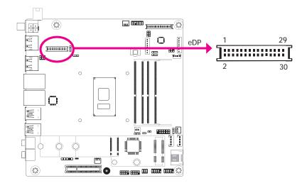
The eDP connector is an embedded displayport which has advanced power-saving features to connect a display device to transmit digital communication of audio and video signals. The table below indicates the pin fuctions of the eDP connector.
