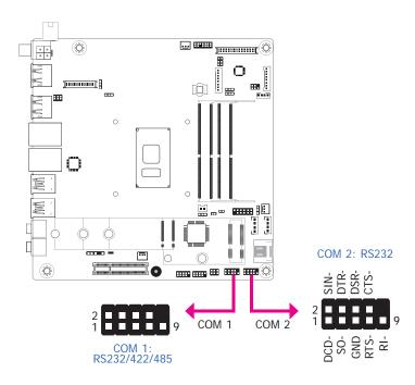
The pin functions of COM 1 will vary according to BIOS' and JP5's settings. COM 1 can be selected among RS232, RS422 and RS485 via BIOS. JP5 is designed to configure Serial COM port 1 to pure RS232 or RS232 with power. Refer to "COM 1 RS232/Power Select" in this chapter for more information.
