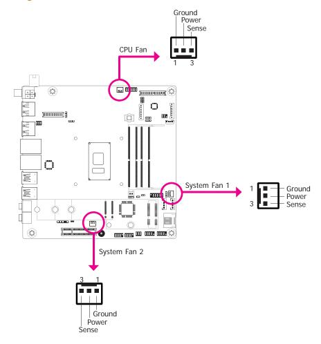
The fan connectors are used to connect cooling fans. The cooling fans will provide adequate airflow throughout the chassis to prevent overheating the CPU and system board components.
