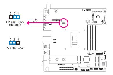
JP3 is used to select the power level of the eDP Inverter power supply.
