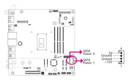
These SATA power connectors supply power to the SATA drive. Connect one end of the provided power cable to the SATA power connector and the other end to your storage device.
