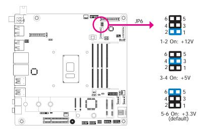
JP6 is used to select the power supplied with the LVDS LCD panel.
