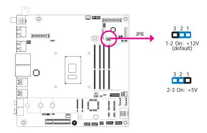
JP8 is used to select the power level of the LCD/Inverter power connector.
