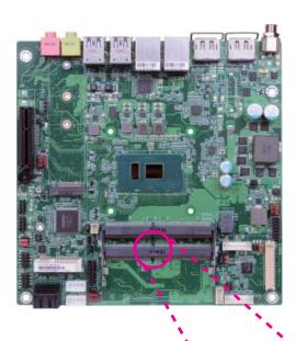
Grasping the module by its edges, align the module into the socket at an approximately 30 degrees angle. Apply firm even pressure to each end of the module until it slips down into the socket. The contact fingers on the edge of the module will almost completely disappear inside the socket.
