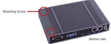
2. Align the mounting holes of the system and the mounting holes on the bracket, and then use the screws removed on step 1 to secure the bracket in place.
