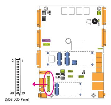
The system board allows you to connect a LCD Display Panel by means of the LVDS LCD panel connector and the LCD/Inverter power connector. These connectors transmit video signals and power from the system board to the LCD Display Panel.
