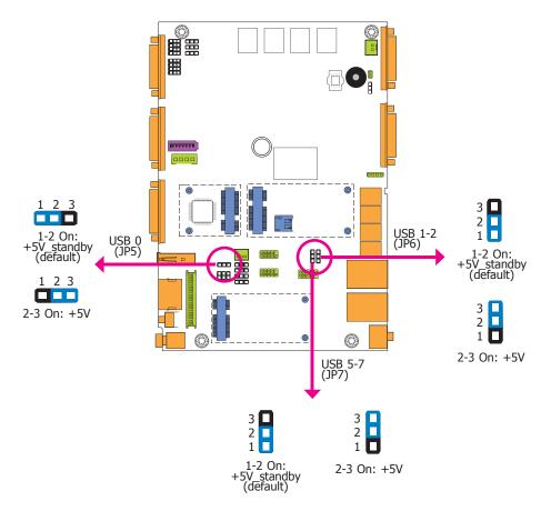
JP5, JP6 and JP7 are used to select the power of the USB ports. Selecting +5V\_standby will allow you to use a USB device to wake up the system.
