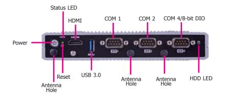
The front panel I/O ports consist of the following:
