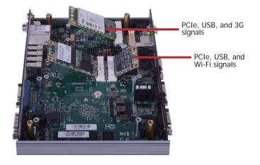
4. Push the Mini PCIe card down and use the provided mounting screws to secure the card on the system board.
