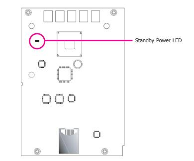
This LED will blink when the system is in the standby mode. It indicates that there is power on the system board. Power-off the PC and then unplug the power cord prior to installing any devices. Failure to do so will cause severe damage to the motherboard and components.
