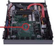
removing the screw on the middle of the motherboard
