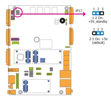
JP17 is used to select the power of DIO (Digital I/O) signal.
