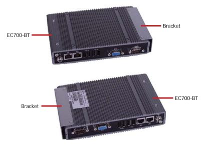
3. The 3 mounting holes on the bracket of the system is used to mount the DIN rail bracket.
