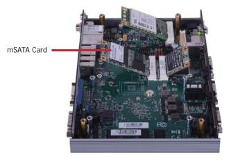
4. Push the mSATA card down and use the provided mounting screws to secure the card on the system board.
