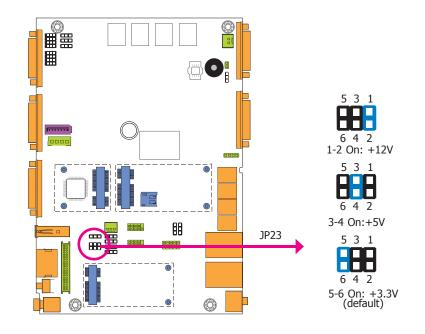
JP23 is used to select the power supplied with the LCD panel.
