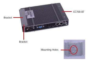
4. Align the mounting holes of the bracket in the system and the mounting holes on the DIN rail bracket, and then use the provided mounting screws to secure the bracket in place.
