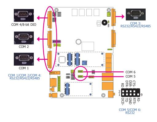
The serial ports are asynchronous communication ports with 16C550A-compatible UARTs that can be used with modems, serial printers, remote display terminals, and other serial devices.
