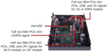
6. The SIM slot is readily accessible after removing the screw on the middle of the motherboard (under the HDD if it has already been installed into the system) and 4 screws on the top side of the chassis cover.
