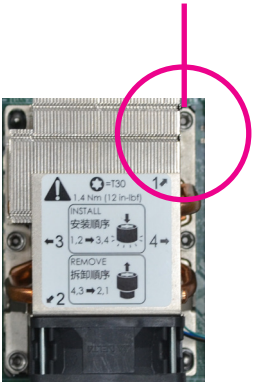
Mounting hole #1 of the heat sink (top view)
