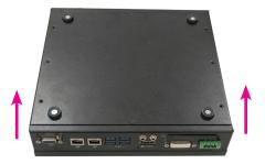
5. The SODIMM sockets, Mini PCIe slot and SATA drive bay are accessible after removing the chassis cover.
