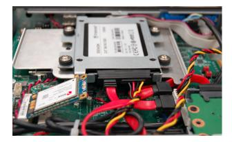
2. Push the Mini PCIe card down and use the provided mounting screw to secure the card on the system board.
